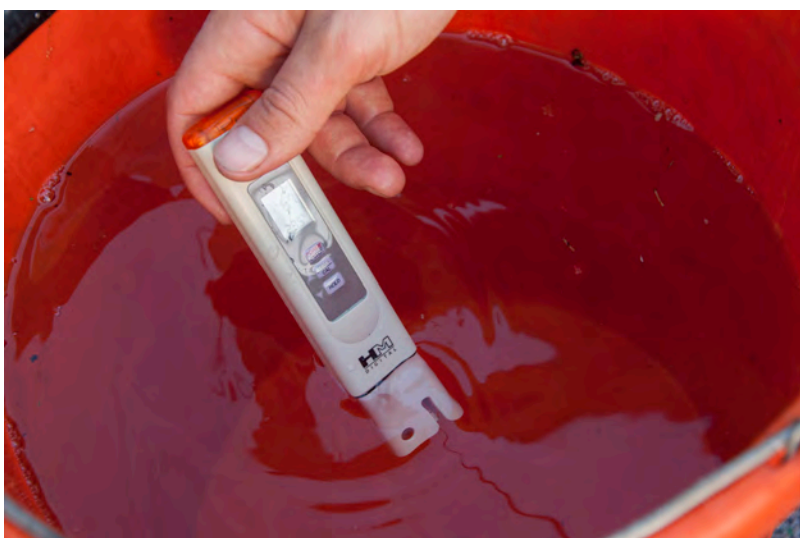
Fig 3.8 Checking the pH Level Using a Digital Meter
