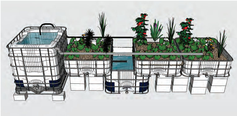
Fig. 4.1-4.5 The Media Bed Method Design
