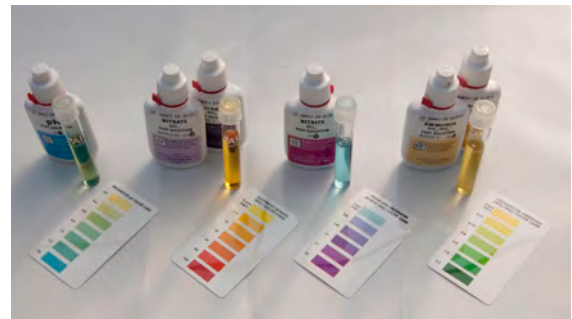
Fig 3.10 Fresh Water Test Kit Set (including tests for: pH, Ammonia, Nitrite & Nitrate)
