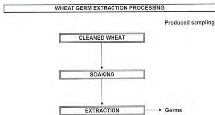
Figure 11 Flow chart of wheat germ extraction processing
