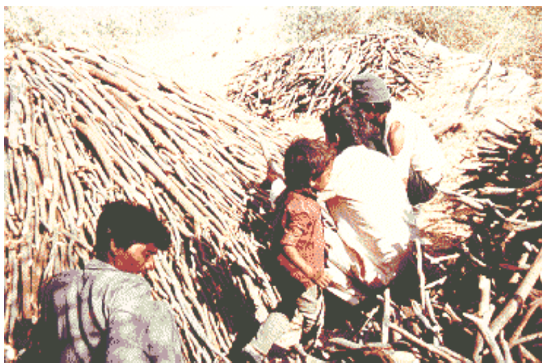
Figure 3.6: Mound Shape Piling of Prosopis Fuelwood for Charcoal Making (by earth mound method)
