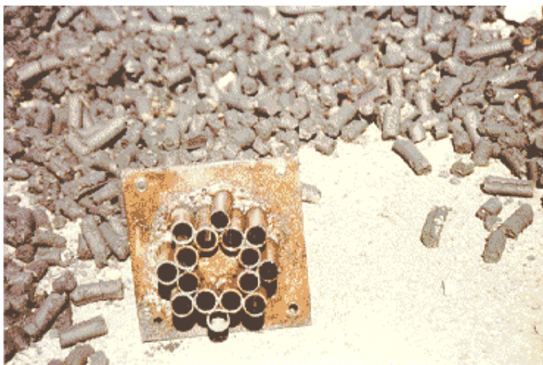
Figure 2.3: Briquette Made from Charcoal Fines, and a Press Mold
