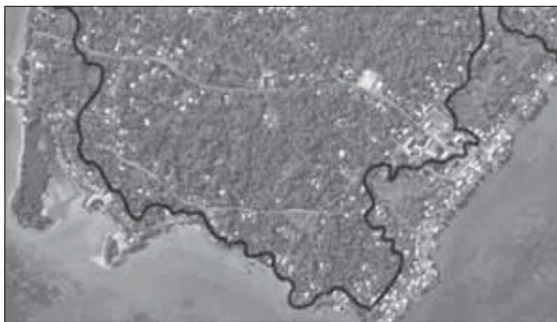
Figure 3 Probable tide limits with an approximate 300 cm sea level rise projection in the populated south of Wallis
