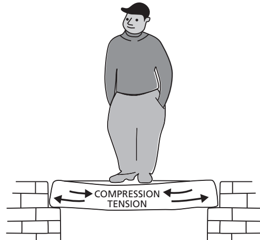
Figure 5.28 Stresses in a concrete lintel
