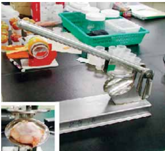
Photo A.2.1 Stainless steel pulper for extracting juice from whole samples. Inset shows a whole cherry tomato after being crushed in the pulper. A small beaker is placed under the sample together the juice extract
