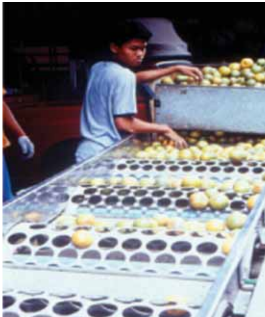
Photo 2.21 Perforated cylinder sizer for citrus makes use of rotating steel cylinders with successively larger openings to classify fruits according to diameter
