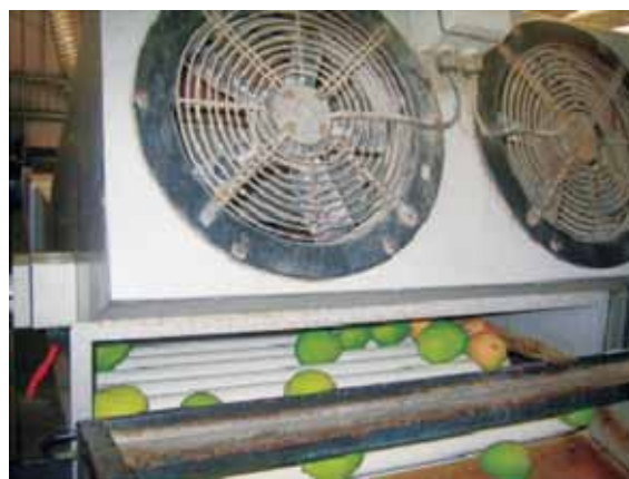
Photo 2.24 An air dryer equipped with blowers and a roller conveyor for evaporating surface moisture from mango fruit
