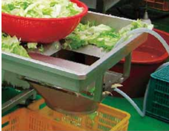
Photo 2.18 A trimming table for fresh-cut lettuce. Note the bevelled corners and rounded edges that minimize the chances for injury to workers and produce. A chute level with the working area and leading to a prepositioned plastic crate under the table is provided for easy disposal of trimmings and rejects
