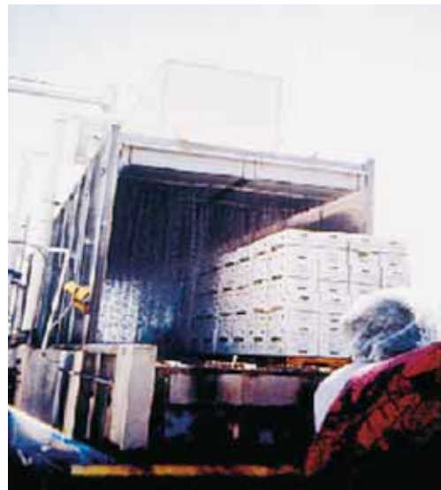
Photo A.3.1 Shower-type hydrocooler for cooling palletized vegetables
