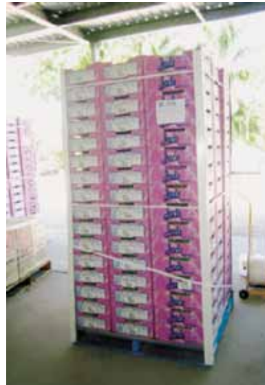
Photo 2.25 Palletized cartons of mangoes with plastic strips fixed to the corners to stabilize the stack
