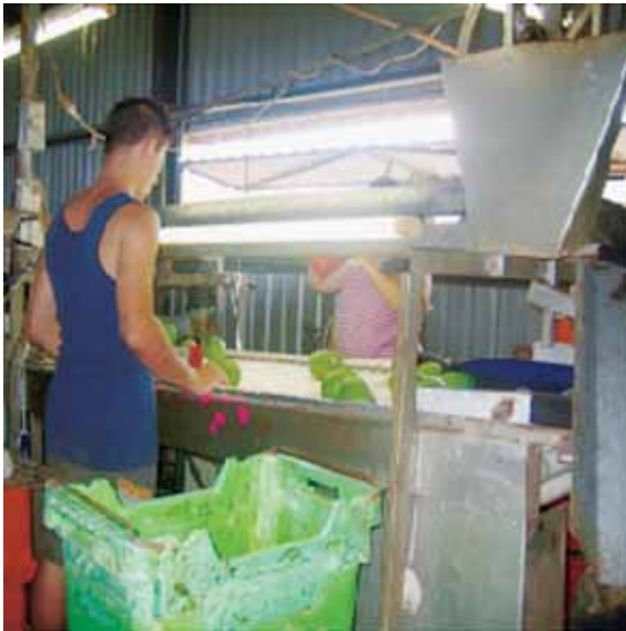
Photo 2.20 A roller conveyor with fluorescent lighting to illuminate the work area while sorters positioned along the sides remove fruit rejects
