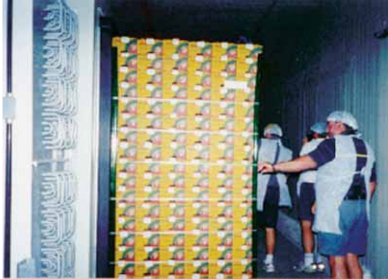
Photo 2.11 Forced air cooling of Brazilian mangoes packed in fibreboard cartons
