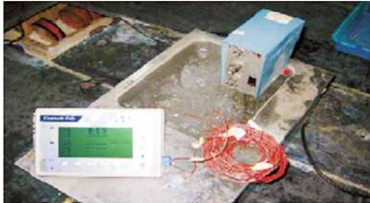
Photo A.5.1 An insulated water bath with water recirculator and ice-water mix for calibration of temperature probes. The recirculator also comes with a heater for controlling temperature of the bath
