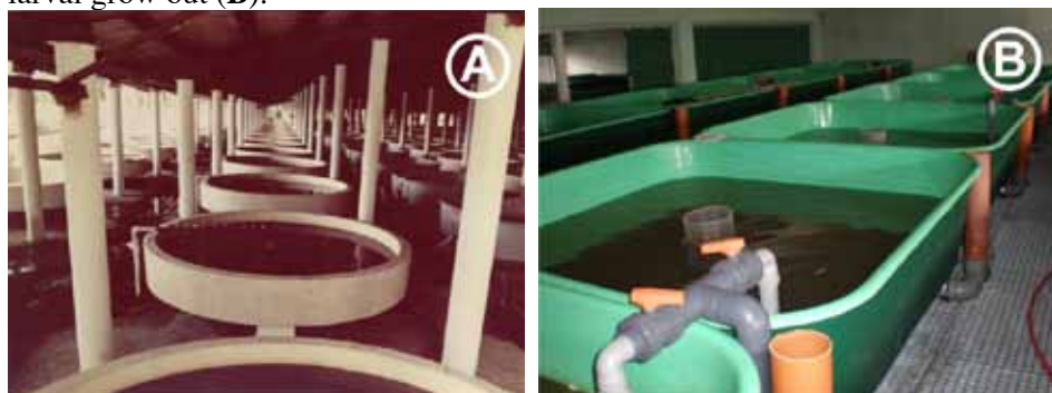
Figure 89: Circular concrete tanks for prelarval holding (A) and plastic trays for larval grow out (B).
