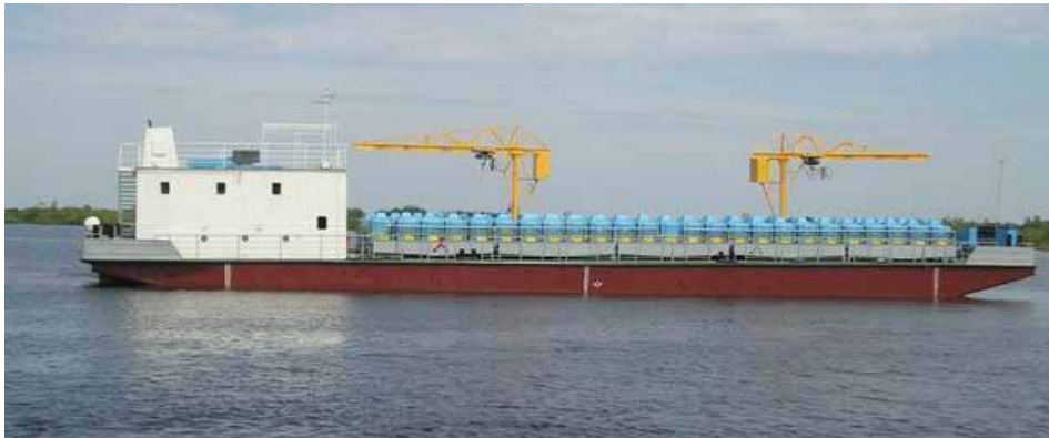
Figure 111: Transportation of sturgeon fingerlings to release sites using a special live-fish vessel (Chepurkina et al. , 2008).
