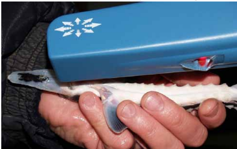
Figure 131: Detection of a coded wire micro-tag with the use of a special detector.
