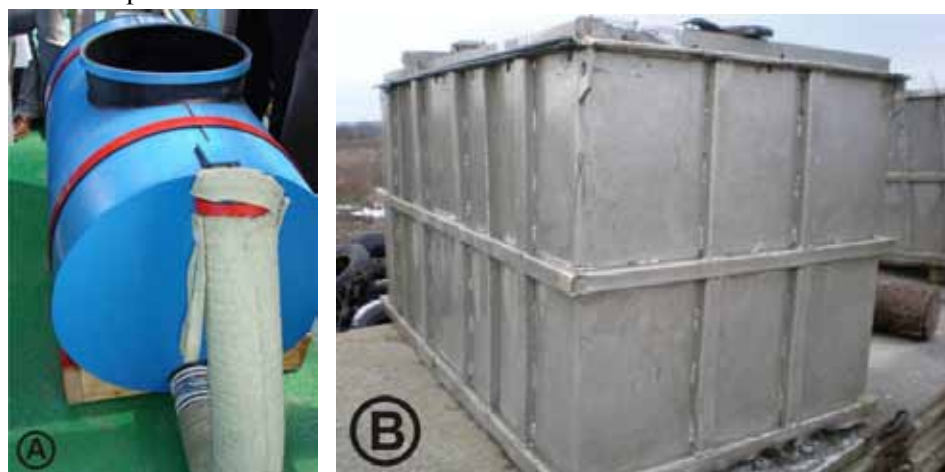
Figure 125: A – loading container for short-term fish transportation (volume = 300 liter) (Chepurkina et al. , 2008); B – specially designed container for short-term transportation of live fish.
