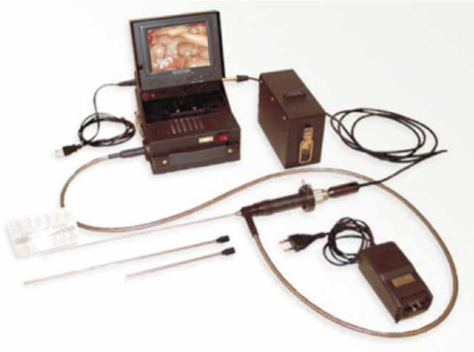
Figure 38: Endoscopic system used for determination of sex and gonadal maturity status.
