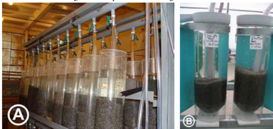
Figure 78: MacDonald jar system: A – incubation jar line; B – separate jars installed in the rearing tanks for prelarval hatching.
