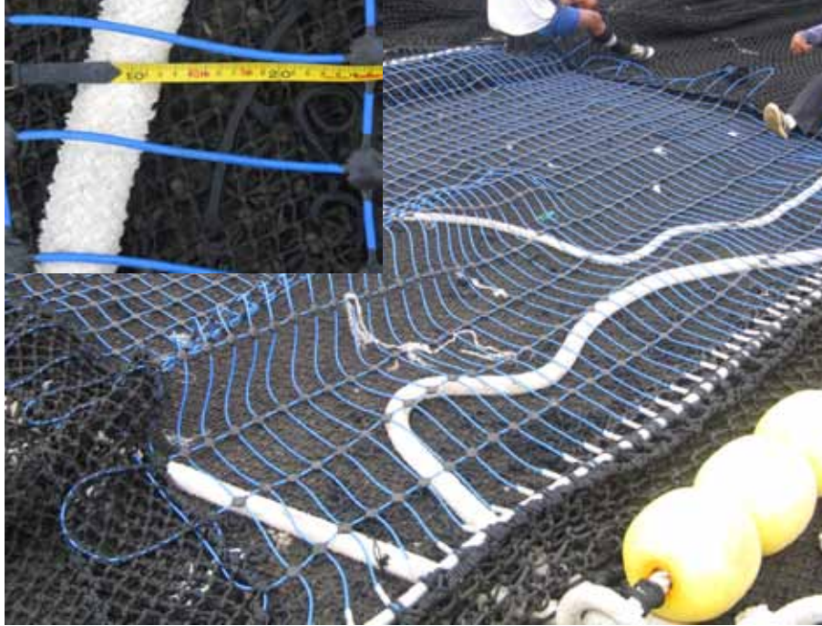
PLATE 4 Arrue's sorting grid – details of construction.
