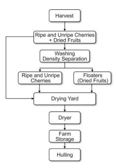
Figure 3. Wet processing flow
