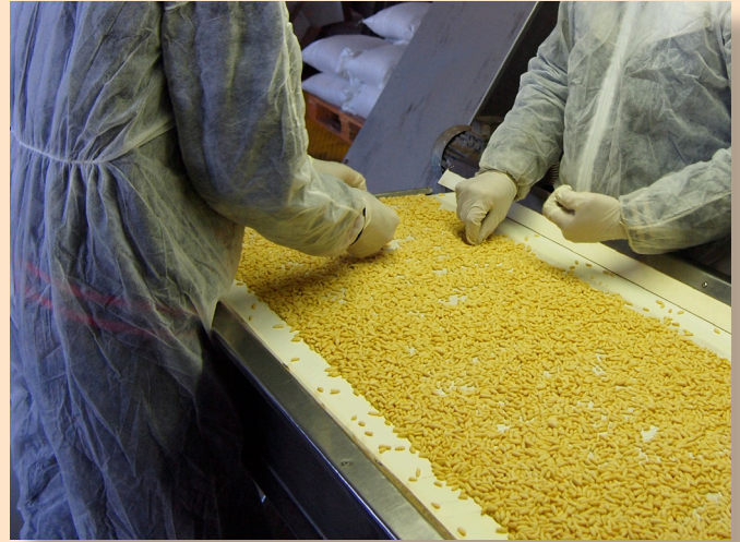
Manual sorting of pine nuts. Appropriate access to and use of personal protective equipment and documented hygiene training programmes are important to prevent contamination of the final product.
