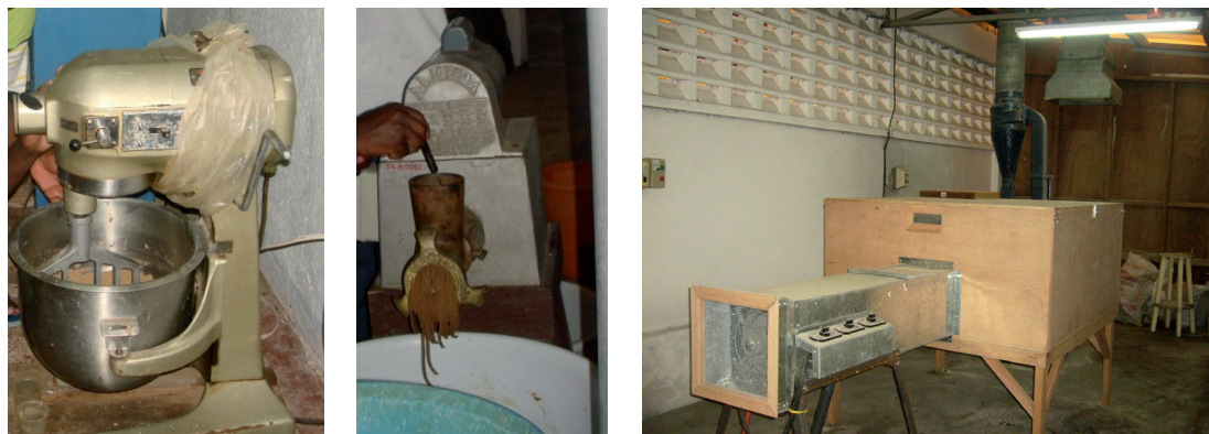
FIGURE 6 Basic equipment used for making farm feeds at SEAFDEC/AQD Binangonan Freshwater Station: feed mixer (left), meat grinder/pelletizer (middle) and fabricated feed dryer (right)
