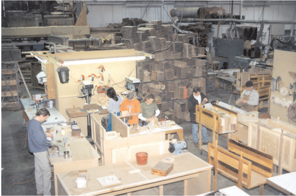
An indoor production area of 6,000 square feet annually transforms 30,000 board feet of lumber into value-added products. Photo by George Hessenthaler
