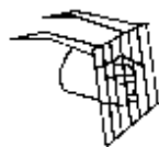
Permanently fixed vermin grating
