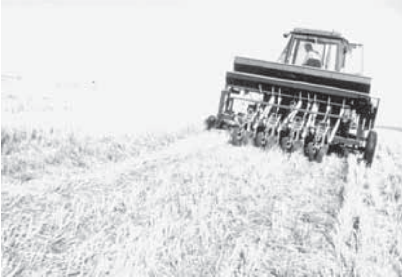
Fig. 5.4. An example of Class IV no-tillage slot cover in heavy standing wheat stubble and scattered straw (from Baker et al. , 1996).
