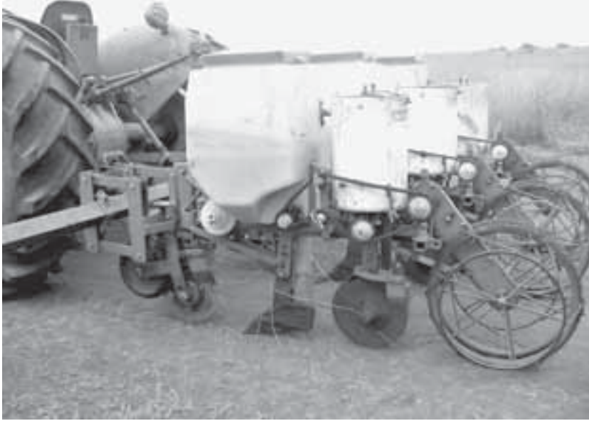
Fig. 14.12. A small planter adapted from animal operation for tractor mounting.
