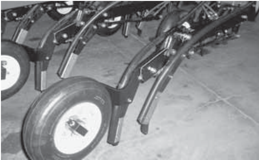
Fig. 4.14. A pair of shank openers with horizontal offset. The front shank applies fertilizer while the rear shank applies seed offset to one side and sometimes shallower.
