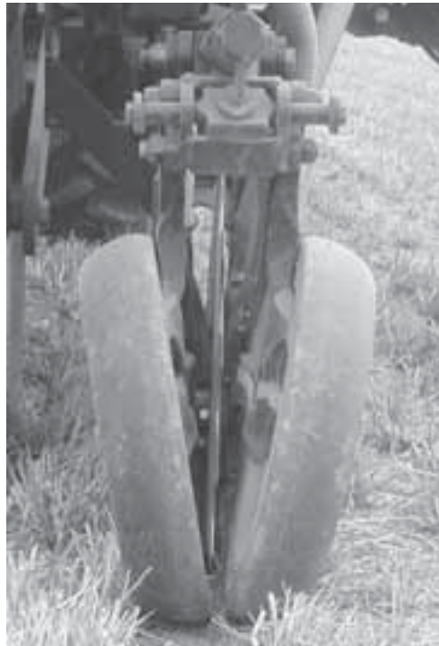
Fig. 8.2. A walking beam arrangement for equalizing the loads carried by two independent gauge wheels.
