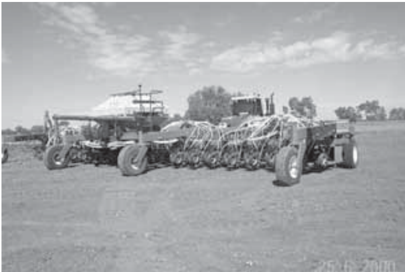
Fig. 13.4. An 18 metre toolbar that is end-towed for transport.
