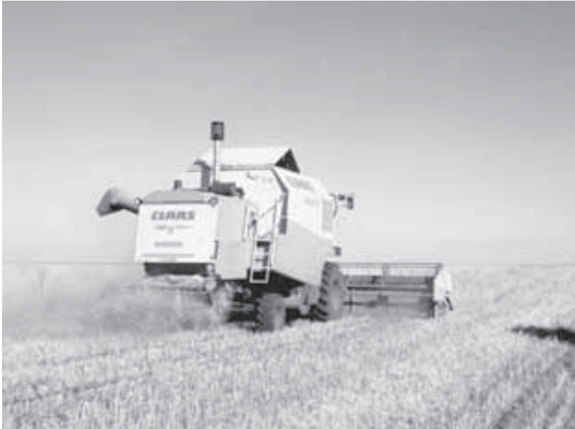
Fig. 10.2. A straw and chaff (tailings) spreader on a combine harvester. Note the dust associated with spreading chaff.
