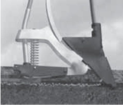
Fig. 5.7. A shank-type opener with packing device to firm seeds into the base of the slot at the same time as covering takes place.
