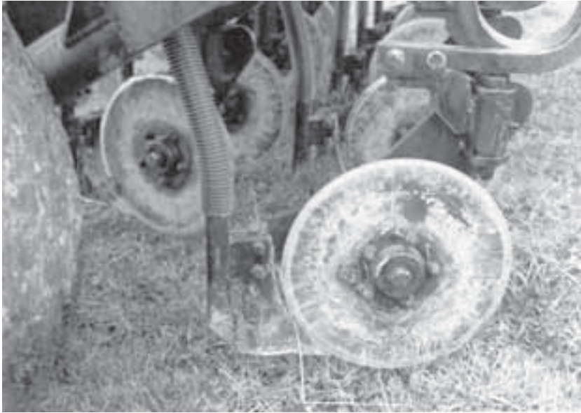
Fig. 4.25. A simple drill featuring a self-steering version of the 'Baker boot' inverted-T-shaped no-tillage opener.
