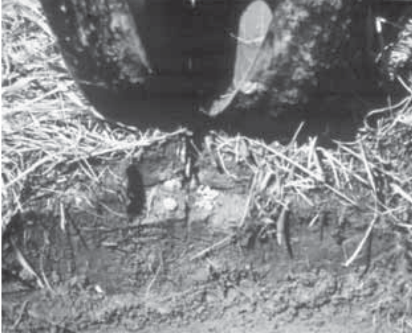
Fig. 9.3. A cross-section of an inverted-T-shaped slot showing the horizontal banding of seed (left) and fertilizer (right) (from Baker and Afzal, 1986).
