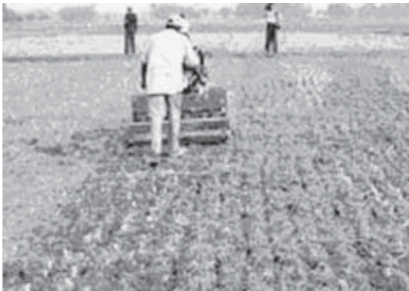
Fig. 14.21. A two-wheeled reduced-tillage machine in strip-tillage mode.
