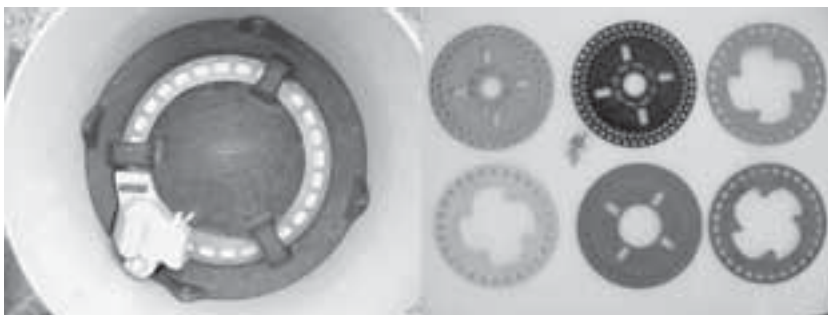
Fig. 14.5. A horizontal plate metering device (left) used in precision planters, with an array of optional seed plates (right).
