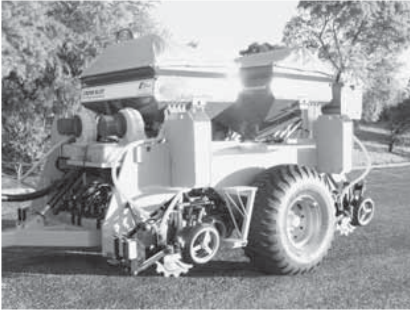
Fig. 8.14. An advanced design of no-tillage air drill.
