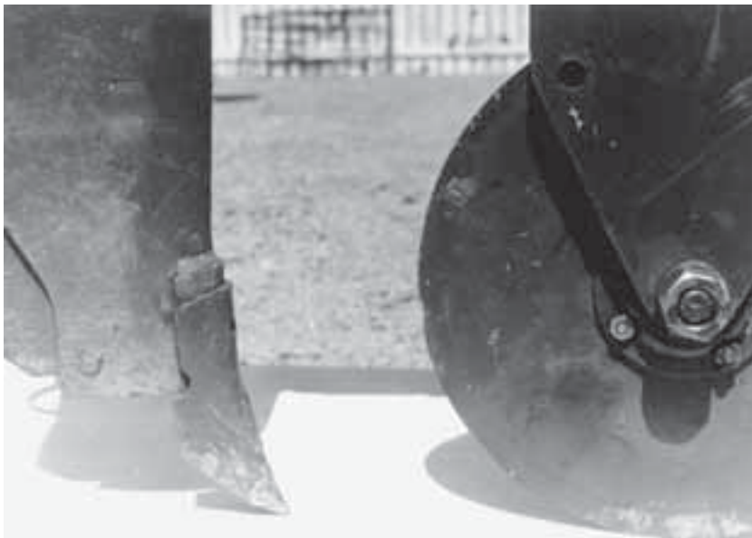
Fig. 4.13. A sharp hoe-type no-tillage opener (from Baker, 1976b).
