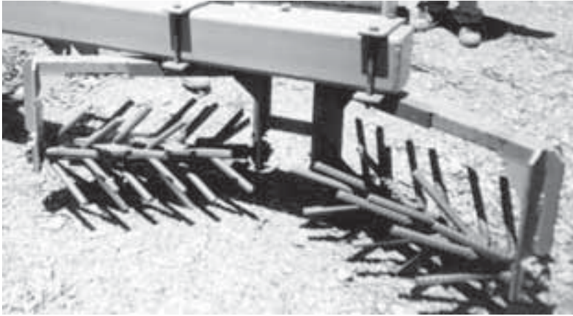
Fig. 16.8. Rolling maintenance tool used to deal with plastic flow of soil out of the wheel ways. This would not normally be used on more than an annual basis (J. Grant, 2001, personal communication).
