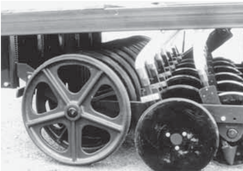
Fig. 4.9. A pair of angled flat disc no-tillage openers (from Baker et al. , 1996).
