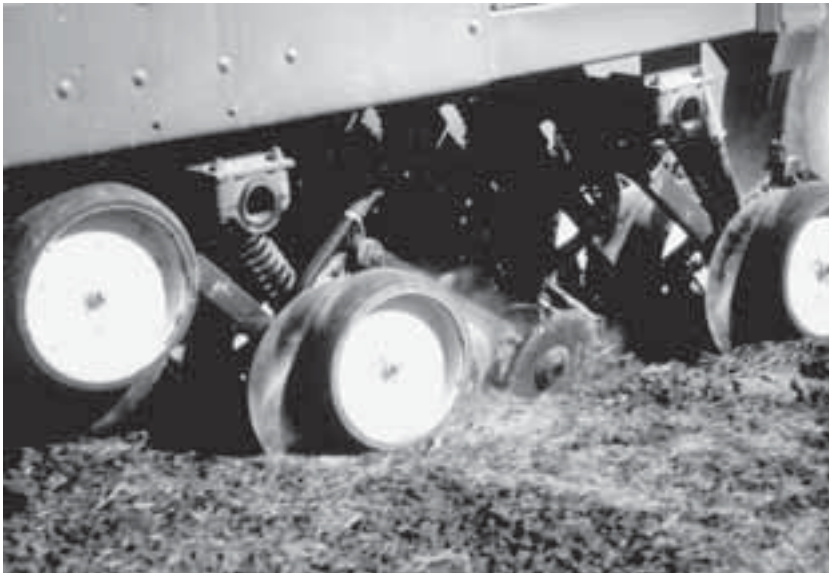
Fig. 8.1. Depth-gauging wheels located alongside the point of deposit of seed in a no-tillage opener.
