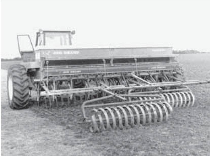
Fig. 5.10. A spiral-caged roller for covering no-tillage slots.
