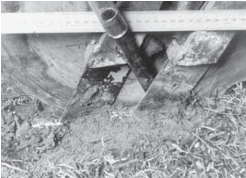
Fig. 9.4. A prototype winged opener with long and short blades for vertical separation of seed and fertilizer (from Baker and Afzal, 1986).
