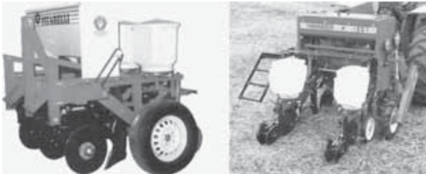
Fig. 14.11. Two small planters with bulk fertilizer hoppers and precision seeders.
