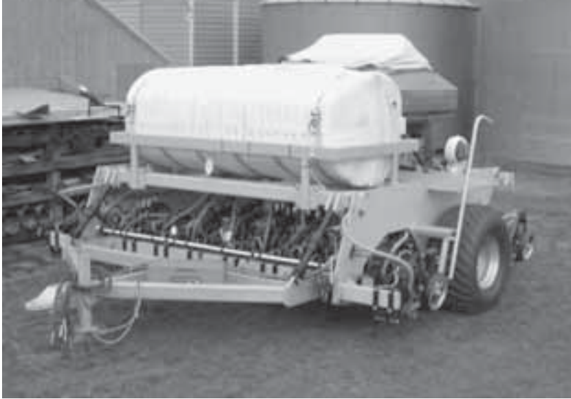
Fig. 13.1. A 4.5 metre wide rigid-frame end-wheel no-tillage drill.
