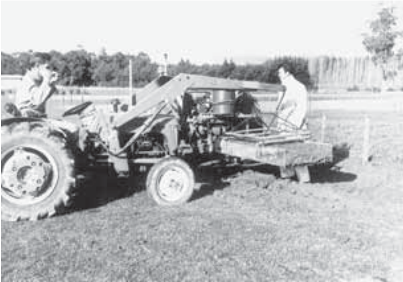
Fig. 19.2. A filled soil bin being transported.
