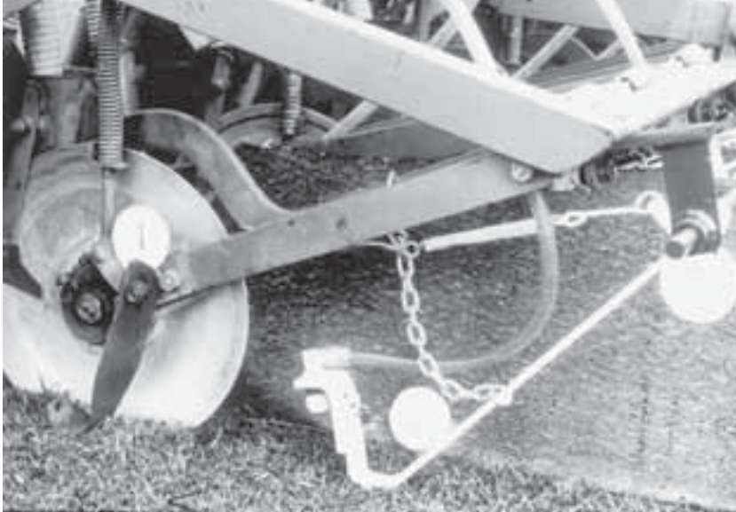
Fig. 12.8. A band spraying nozzle mounted on separate skids to control spraying height.
