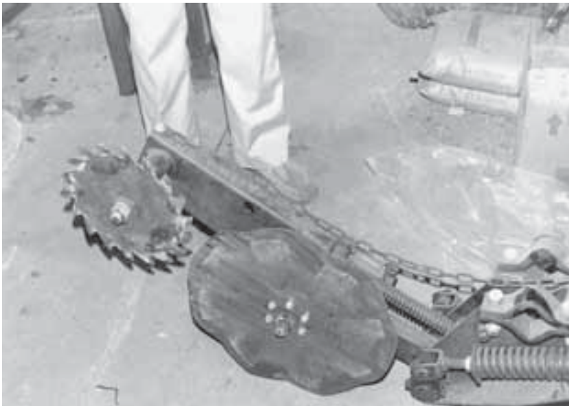
Fig. 4.19. A power till no-tillage opener driven by a ground-engaging wavy disc (from Baker et al. , 1996).
