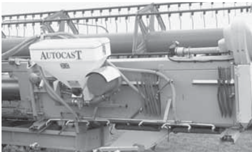
Fig. 4.31. 'Auto-casting' of seed behind the pickup table of a combine harvester.
