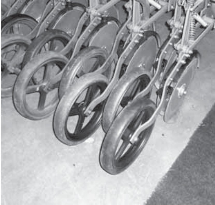
Fig. 4.2. Typical offset double disc no-tillage openers that create vertical V-shaped slots.
