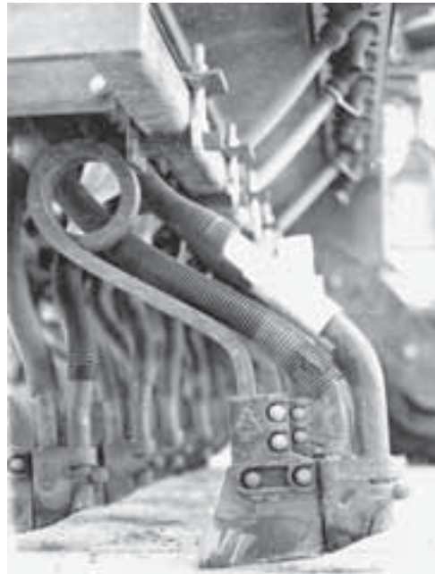
Fig. 4.24. A simple drill featuring 'Baker boot' inverted-T-shaped no-tillage openers (from Baker et al. , 1996).
