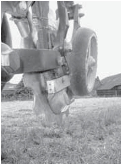
Fig. 4.27. A disc version of the winged opener for creating inverted-T slots.
