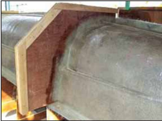
Figure 64 Mould framework. The shape of the frame is for tilting of the mould (See Figure 80)
