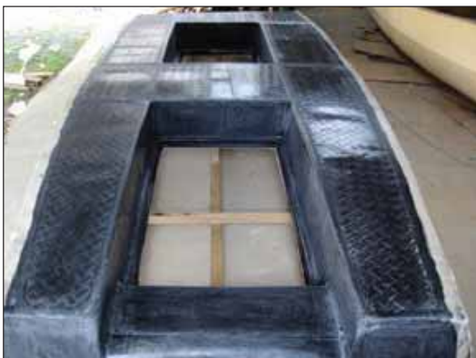
Figure 108 Cockpit deck mould complete.
