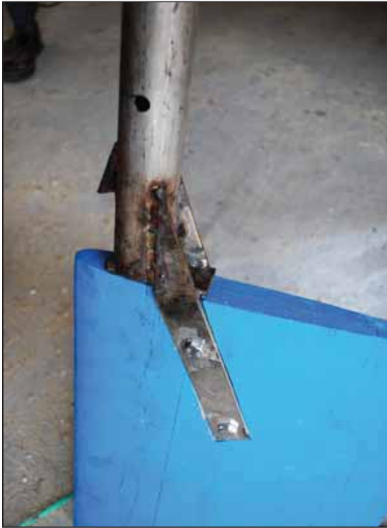
Figure 120 Detail of the rudder for the BOB-drive.
