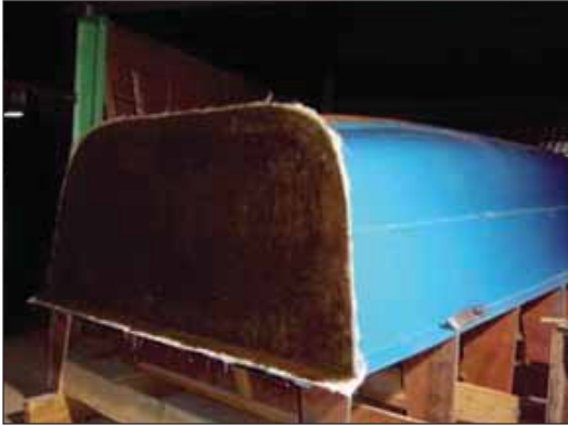
Figure 59 Transom lay-up completed.
