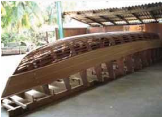
Figure 46 Applying veneer ply skin.
