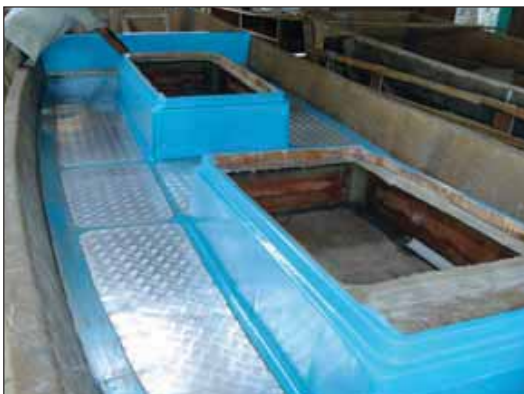
Figure 107 Note the metal plates on the deck to prevent a slippery surface.
