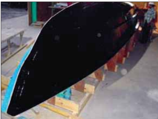
Figure 61 Gelcoat on starboard half.
