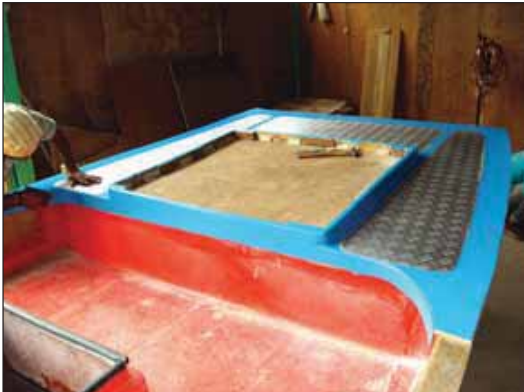
Figure 117 The engine hatch coaming on the aft deck plug.
