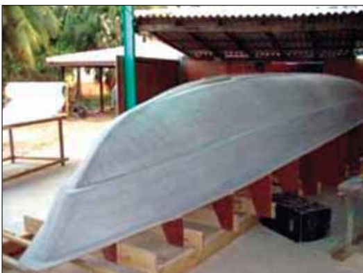
Figure 52 Hull plug ready for painting.
