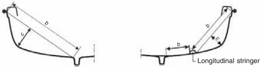
BOAT WITH CURVED BOTTOM AND KEEL + TRANSVERSE FRAMES SPACED MORE THAN b
