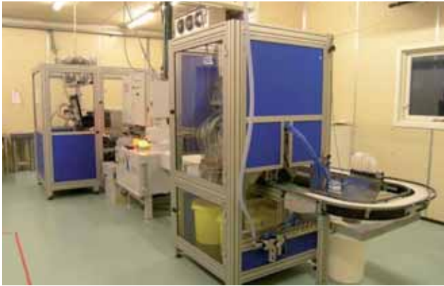
Fig. 1 Real-Time Sorting Machine using X-rays and Image Analysis (Source: Incotec International BV)
