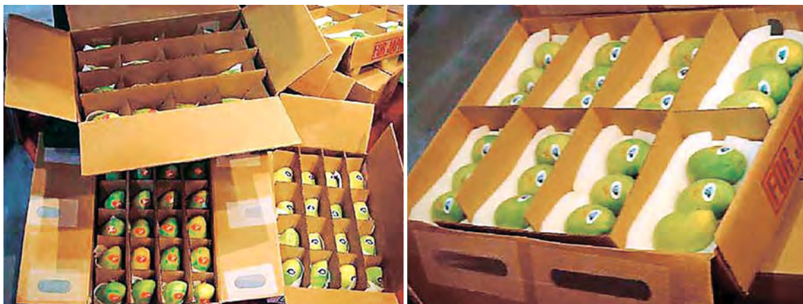
17 kg; 200-test, partitioned, wet-strength boxes, with ventilation holes covered with nylon mesh, with or without foam padding for the packaging of vapour heat treated mangoes.
