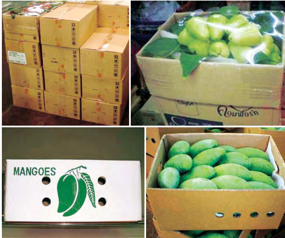
Regular slotted container (RSC) (top) and telescope boxes (bottom)
