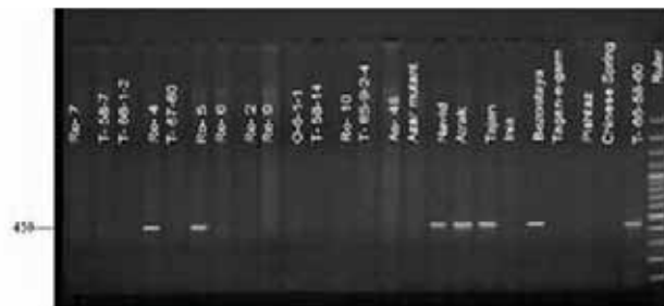
Figure 2 PCR product by P5P6 primer, this primer represent DX5, the genotypes that carrier this subunit produced a 450 band, while other genotypes that have DX2 didn't produce any band.
