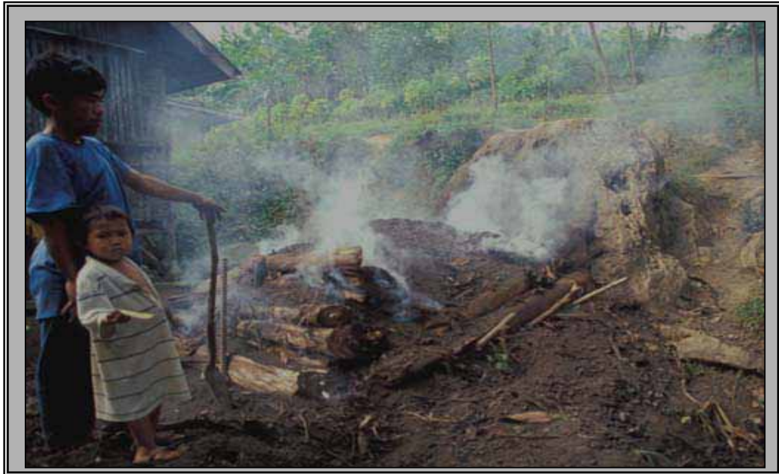
Figure 6. Charcoal maker using the tinabonan method (Underground approach) Barangay Pamutan, Cebu City (Bensel Terrence, 2003).
