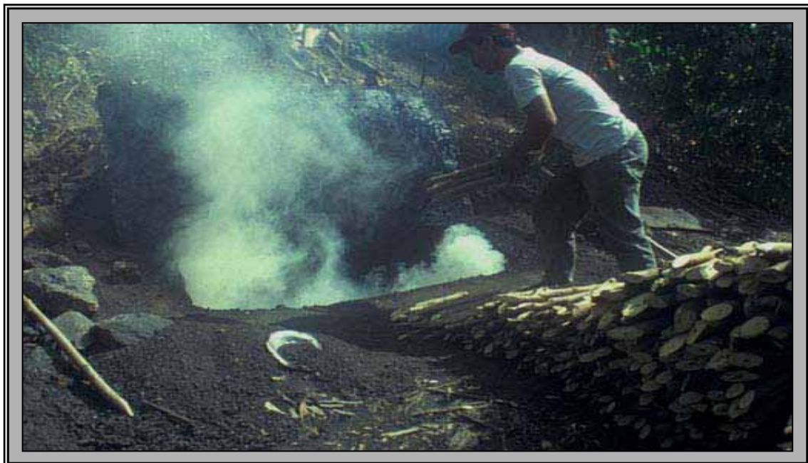
Figure 6. Charcoal maker using the tinabonan method (Underground approach) Barangay Pamutan, Cebu City (Bensel Terrence, 2003).
