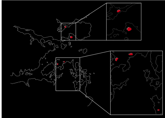
FIGURE 8.5c GIS based particulate dispersion model for Loch Erisort and Loch Leurbost Fjord systems using maximum surface current speed as the forcing image and with a resolution of one metre.
