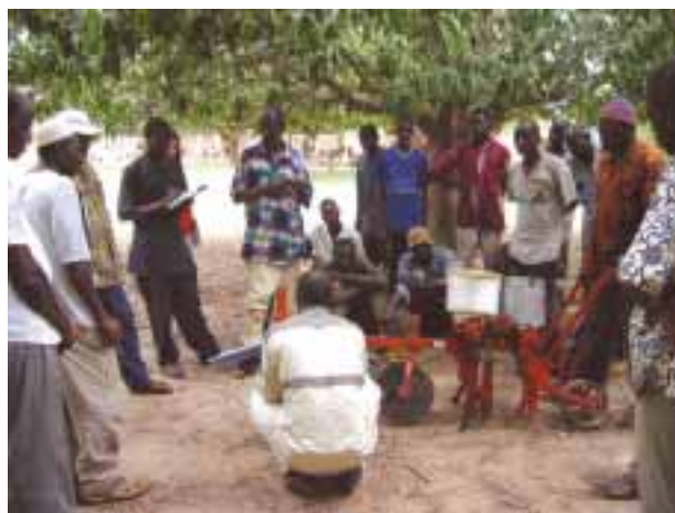
FIGURE 11 Direct seeder (animal drawn) imported from Brazil
