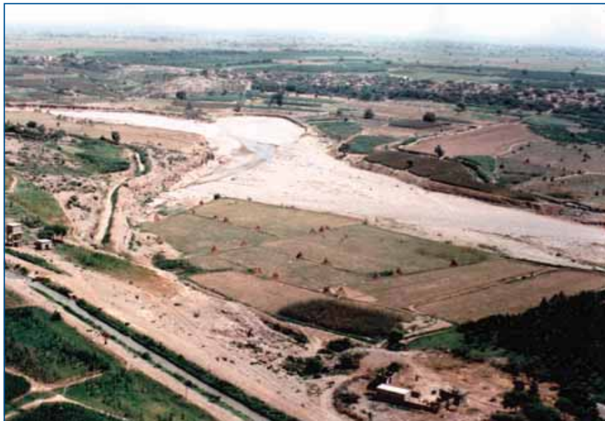
FIGURE 4.25 Bank cutting and the development of a meander, Wadi Rima, Yemen
