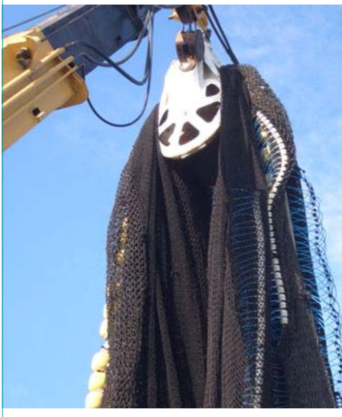
PLATE 3 Flexible sorting grid going through the power block.
