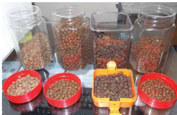
Samples of different sizes of extruded pellets for rainbow trout produced by an industrial feed mill in Bishkek, The Kyrgyz Republic
