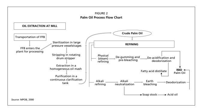
reduced pressure (2–6 mm Hg). Normally, the refinery mixes all the distillates, irrespective of whether from refining of CPO, crude palm olein or crude palm stearin (Figure 2). The final product is generally called PFAD. It is a light-brown solid at room temperature, melting to a brown liquid on heating.
