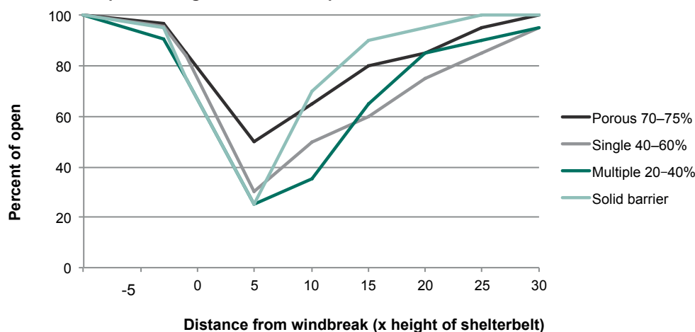
FIGURE 11.4 The effects of windbreak porosity on windflow at different distances from the windbreak for porous, single-row and multiple-row conifers and for a solid barrier
