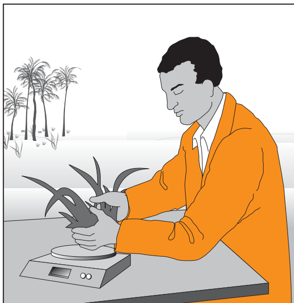
Figure 34. Always take the exact sample size (fresh weight for solid samples and volume for liquid ones) directly after sampling.
