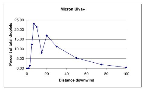
Note: results beyond 50m for the Micron Ulva+ are extrapolated due to no data
