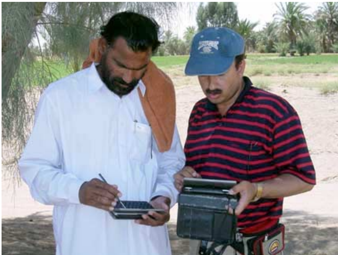
12. Team Leaders used eLocust (a custom database and mapping program on a handheld computer) to record field data. This dramatically improved reporting quality and timeliness.
