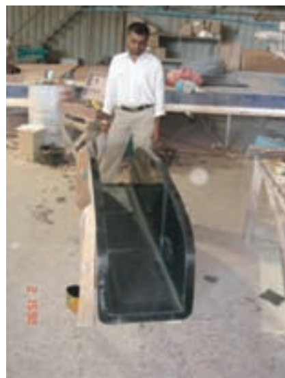
A finished mould for the centre thwart. All the separate parts (structurals and other items) of the boat need their own mould.
