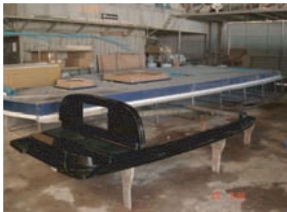
The deck mould ready for use.
