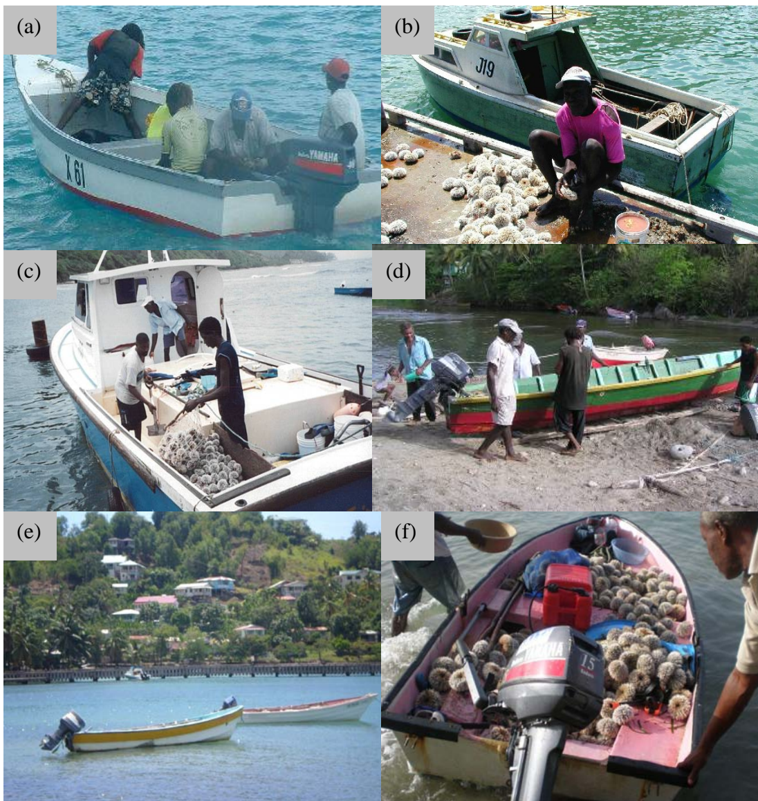
Plate 7: Types of boats used in the harvest of white sea urchins in the eastern Caribbean: (a) small open boat (“moses” in Barbados) with outboard engine; (b) dayboat (Barbados); (c) iceboat (Barbados); (d) dugout canoe with outboard engine (Grenada and Saint Lucia); (e) wooden pirogues with outboard engines (Grenada, Martinique and Saint Lucia); and (f) small open boat with outboard engine (Saint Lucia) [(a) Franklin, (b) Parker, (c) Pena, (d) authors collection, (e) and (f) Cox].
