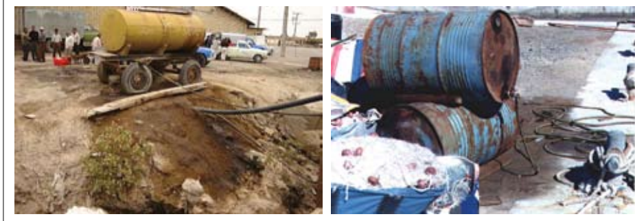
FIGURE 25 Examples of improper storage of fuel
