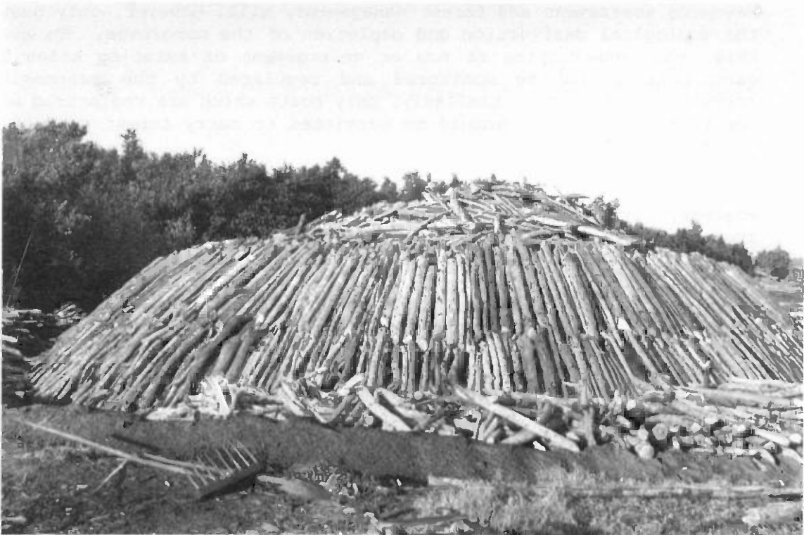
Figure 3.2: Charcoal making by the earth mound method in Guanabacoa, Cuba. Photo by P.W.Chong
