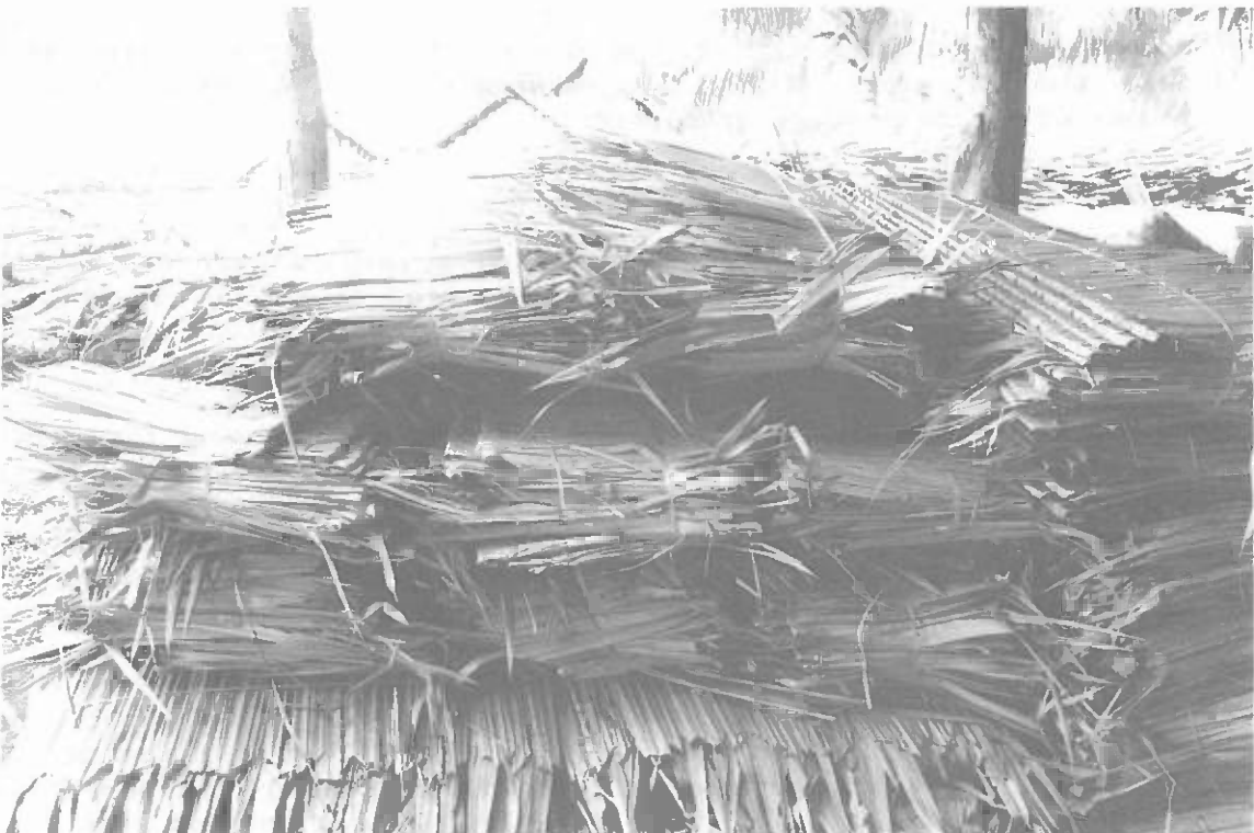
Figure 3.6: Shingles (Atap) made from Nypa leaves in Sumatra, Indonesia. Photo by M.L.Wilkie
