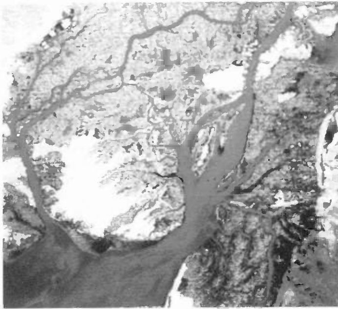
Fig. 5.4: A partial view of a False Colour Composite obtained from combinations of ratios 5/4, 5/7 and 6/5 of Landsat MSS bands. The mangrove appears as orange-red, marsh vegetation as reddish black, shrubs as yellow, crops as bright red and saline areas as white. (Gulf of Kachc Landsat Data, India, 1982) (Courtesy: Nayak)
