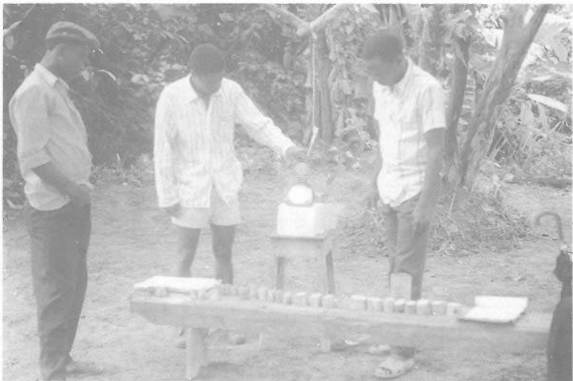
Figure 5.4: Measuring the green density of wood samples, Ma-swar, Sierra Leone Photo by M.L.Wilkie
