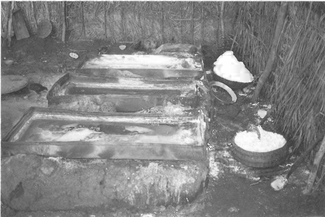
Figure 3.18: Boiling of the brine solution in big pans, Sierra Leone Photo by courtesy of M.P.Wilkie
