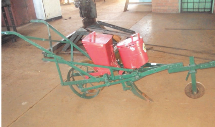
FIGURE 6 A conventional planter which has been adapted to CA through the addition of a cutting disc
