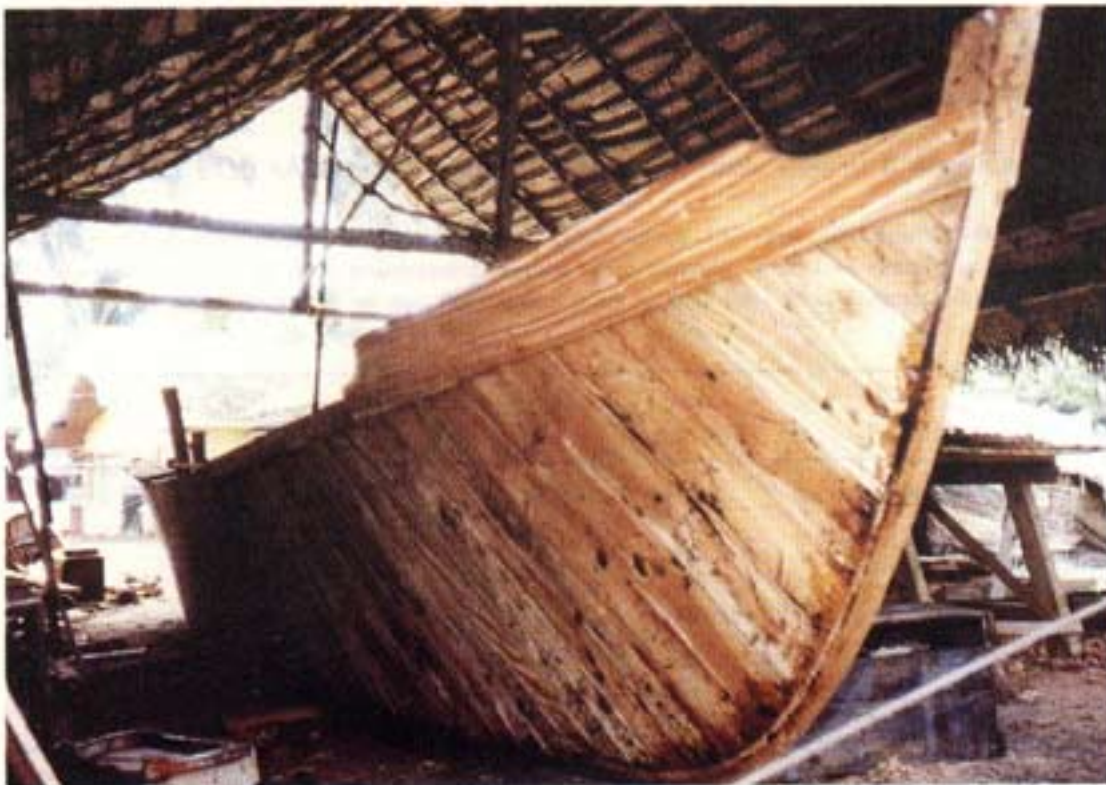
Construction of SRL-18A wooden canoe in Doddanduwa above and below)
