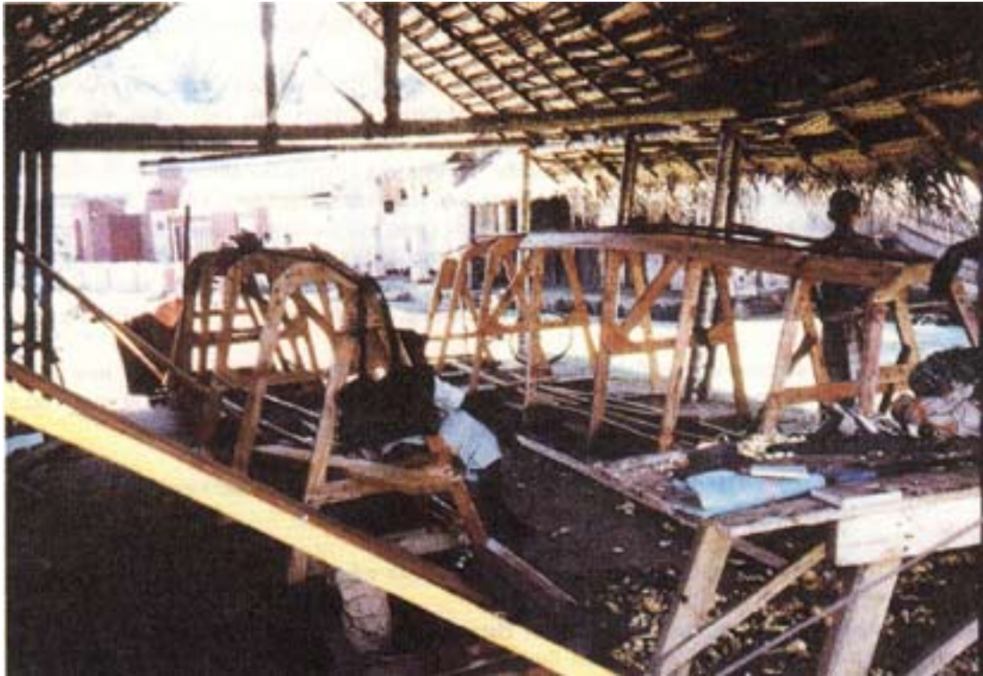
Construction of SRL-18A wooden canoe in Doddanduwa above and below)
