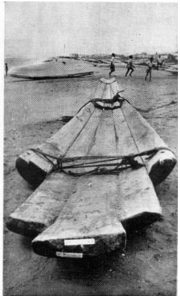
A new assembled unit of kattumaram (five logs) waiting to be launched.
