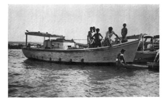
The photographs shown here were used for the fishing gear improvement project. Top: The 28-feet-lon9  $3\frac{1}{2}$ -tonnemade of fibreglass reinforced plastic and fitted with a 33-H.P. engine, that was used in Beruwela.
