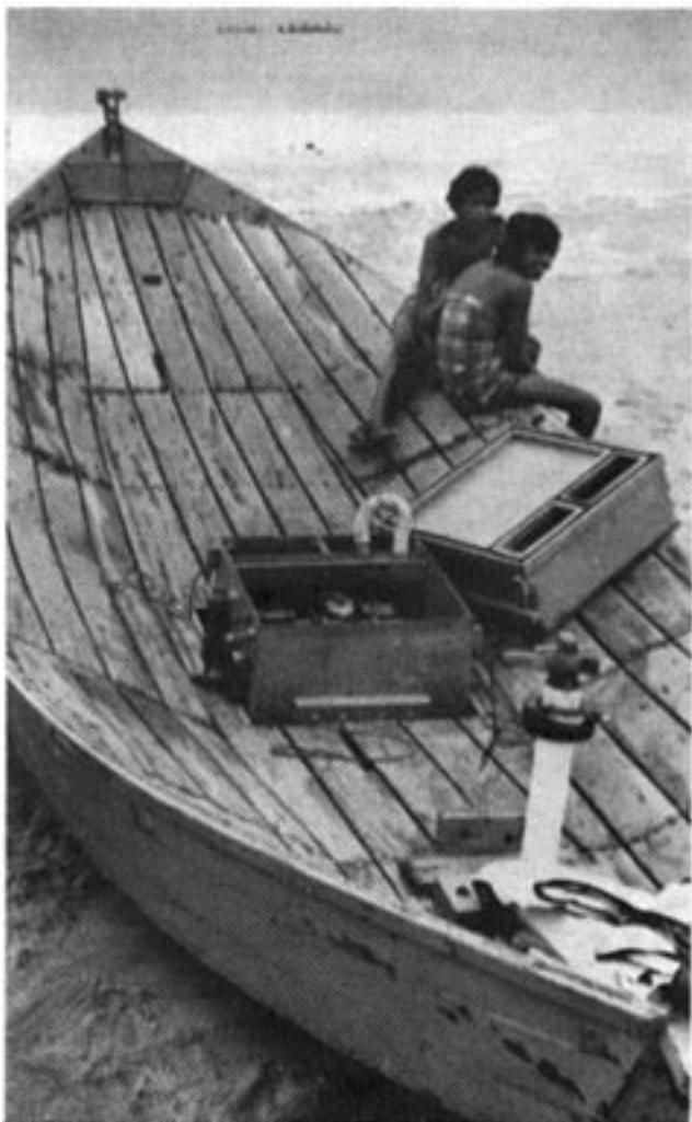
Engine box installed in IND—11. Lid removed. Note Inlet and outlet ports in lid.
