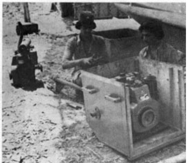
Engine box with forward face and lid removed. Note pivot attached to side.
