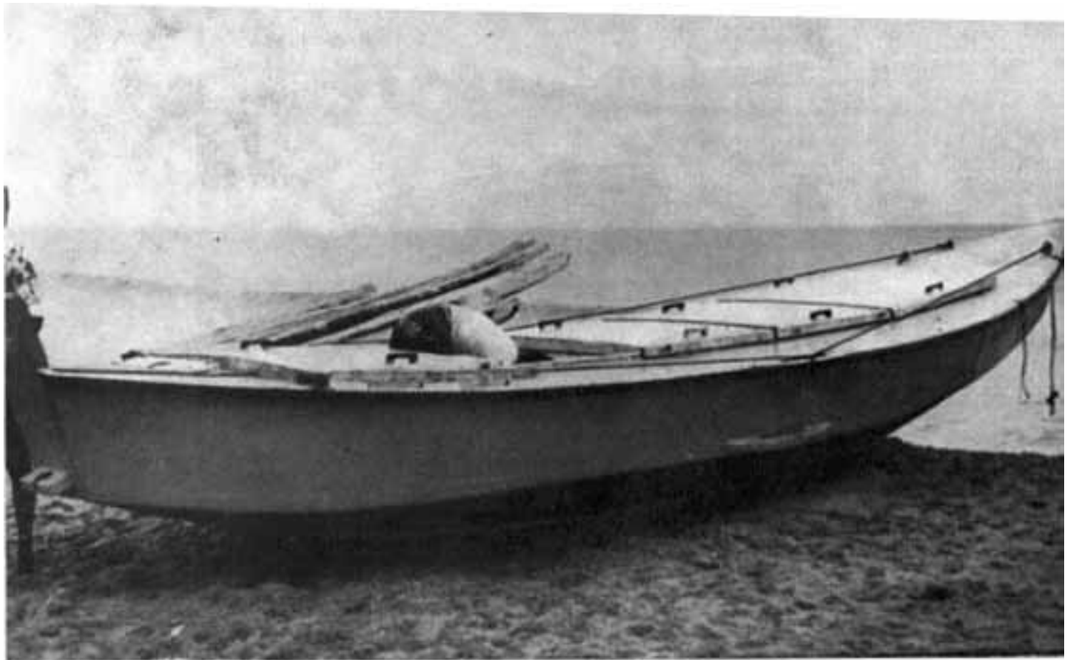
IND-13 (above): 7.40 m long. Decked, built of marine plywood. Equipped with sail and 5 hp inboard engine. One of the two prototypes selected for intensive fishing trials.
