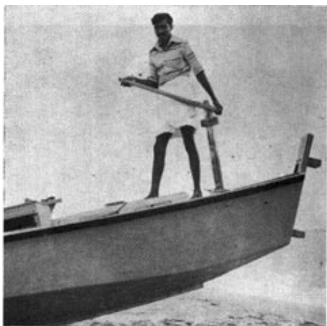
Propeller and rudder in up position.
