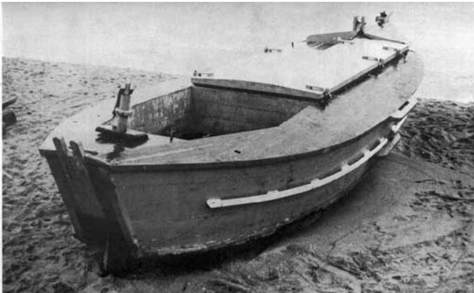
IND-10 (above): 7.02 m long. Decked, made of teak, equipped with sail and 5 hp inboard engine.
