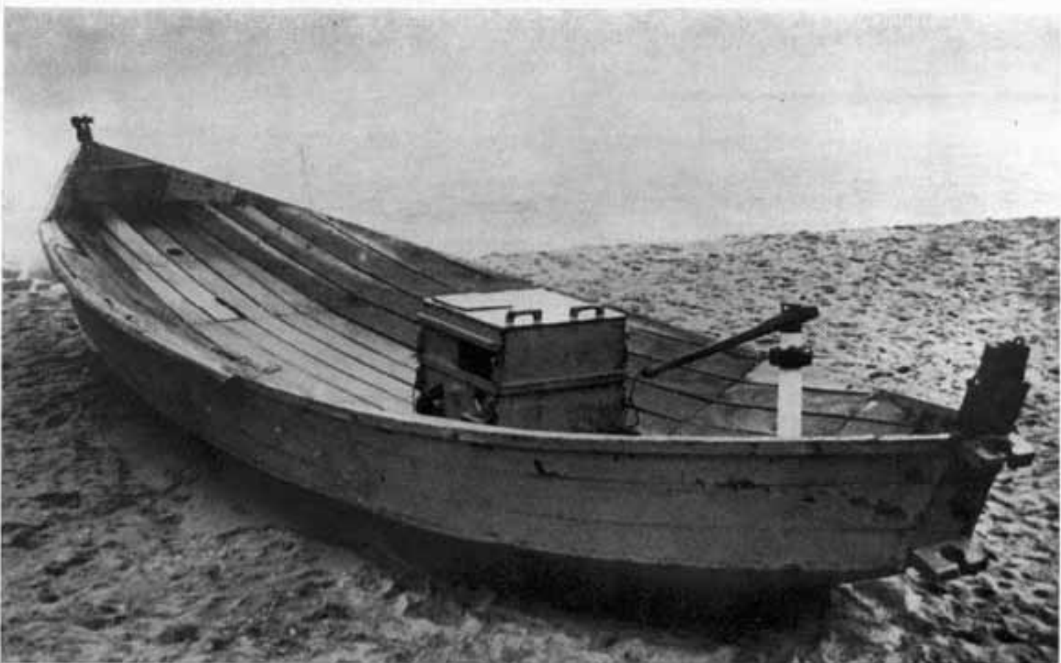
IND-11 (below): 7.40 m long. Uses polystyrene logs enclosed in a non-watertight framework. Equipped with sail and 5 hp inboard engine. One of the two prototypes selected for intensive fishing trials.
