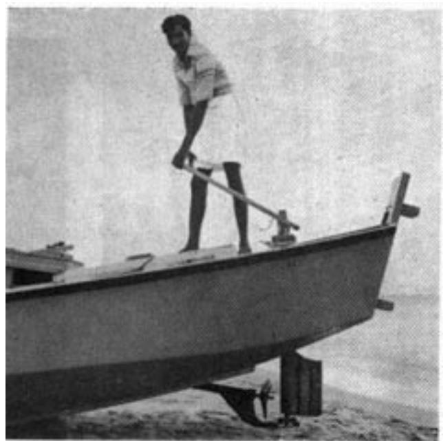
Propeller and rudder in down position.
