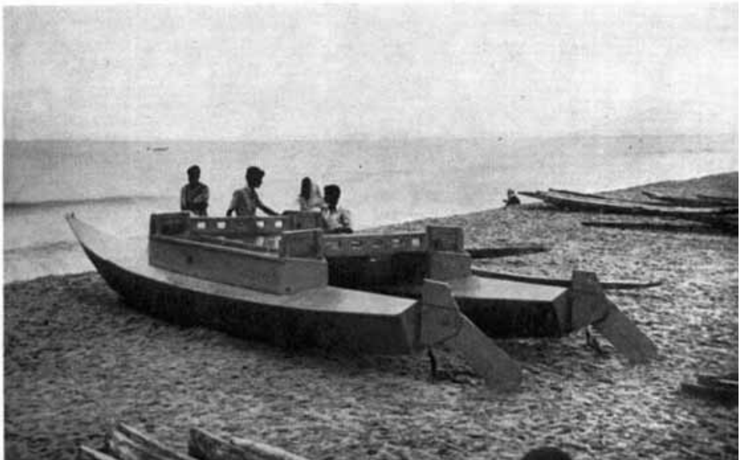
IND-14 (below): 7.20 m long. Twin-hull craft built in marine plywood. Hulls decked forward and aft.
