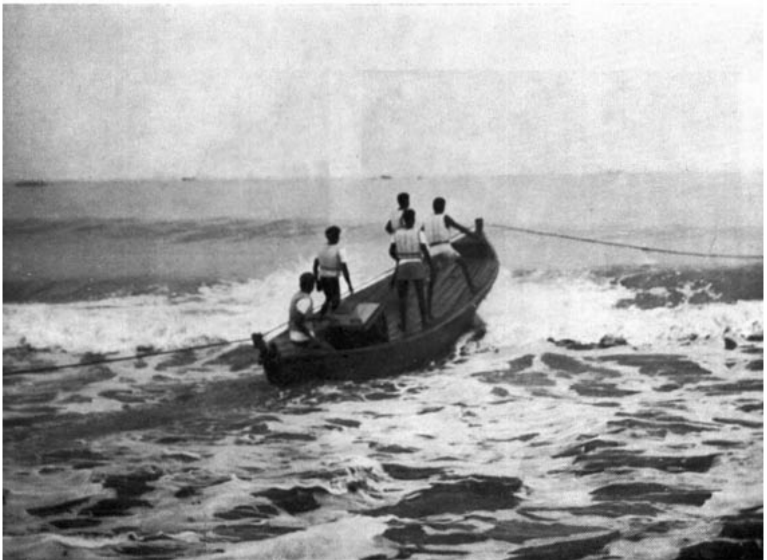
IND-11 using the rope system to cross the surf. Note fore and aft rope fairleads with locking arrangement.
