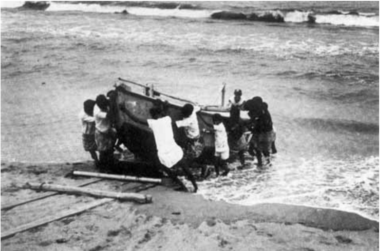
Planks and rollers (above) are placed beneath a BOBP craft for hauling. Note the steepness of the beach. Below: A capstan in operation.
