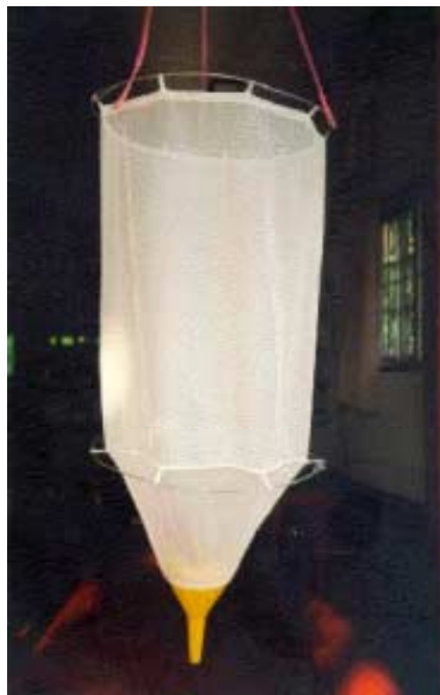
Figure 16. 'Orlon' hatching cone (Note: water flow enters through the funnel in the bottom)
