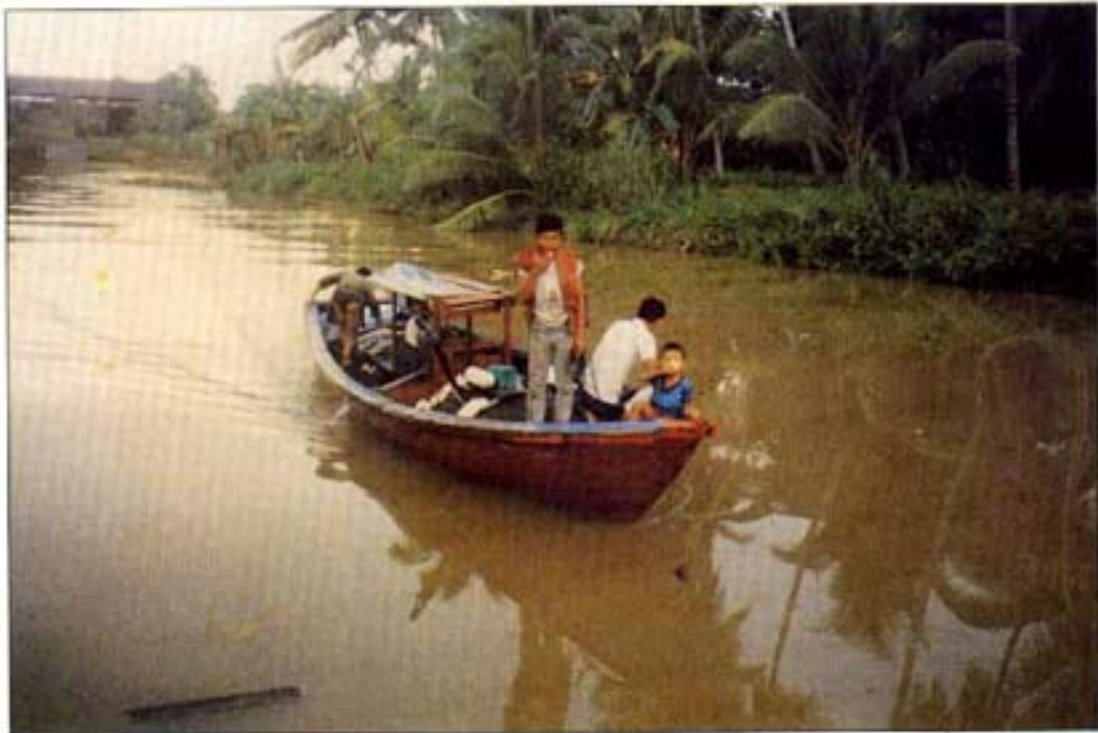
A larger inboard motorized half-deck driftnetter (10-12 m)
