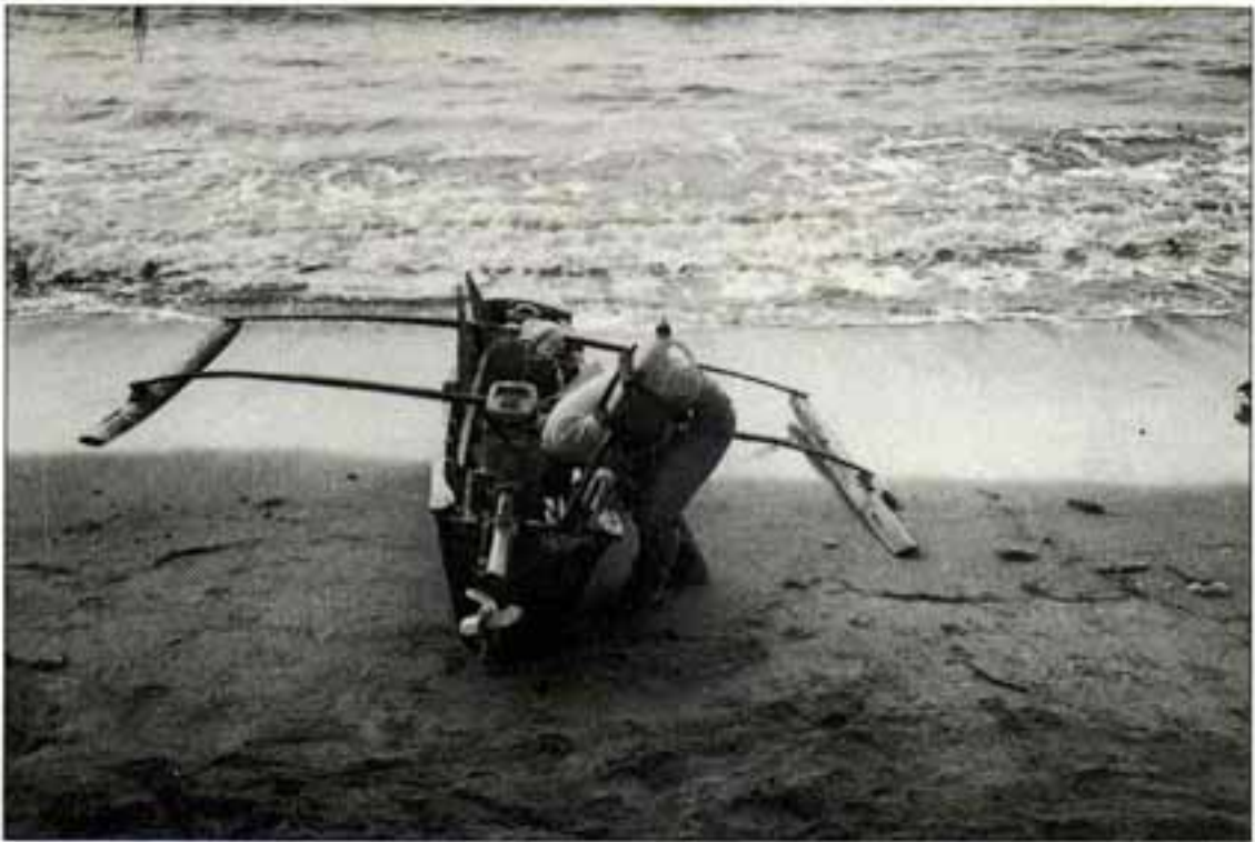
Outboard motorized dugout outrigger canoe (4-5 m)
