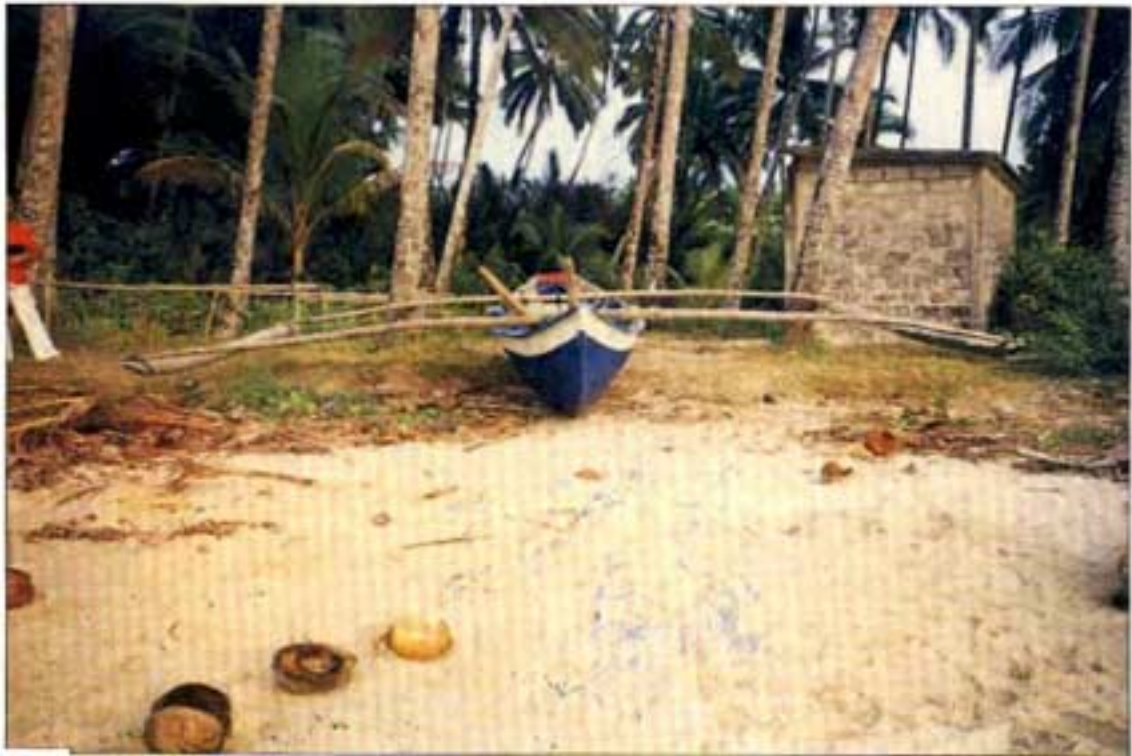
Outboard motorized dugout outrigger canoe (6-7 m) used for beach-seining
