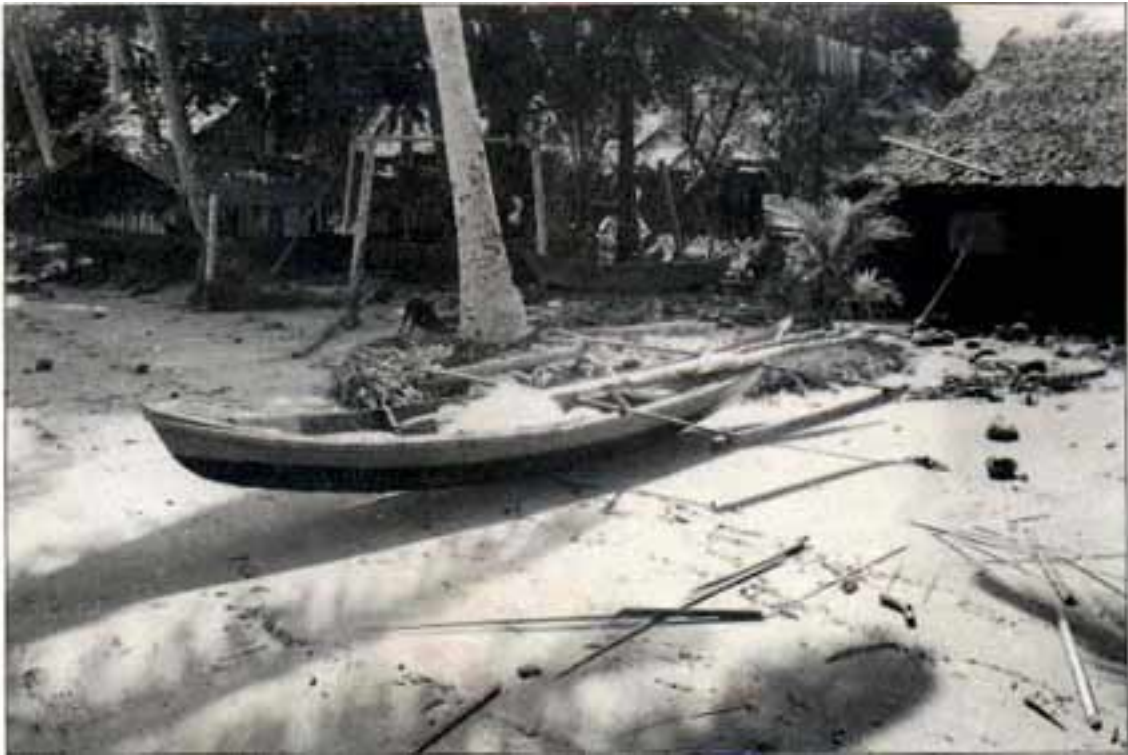
Non-motorized dugout outrigger canoe (4-5 m)
