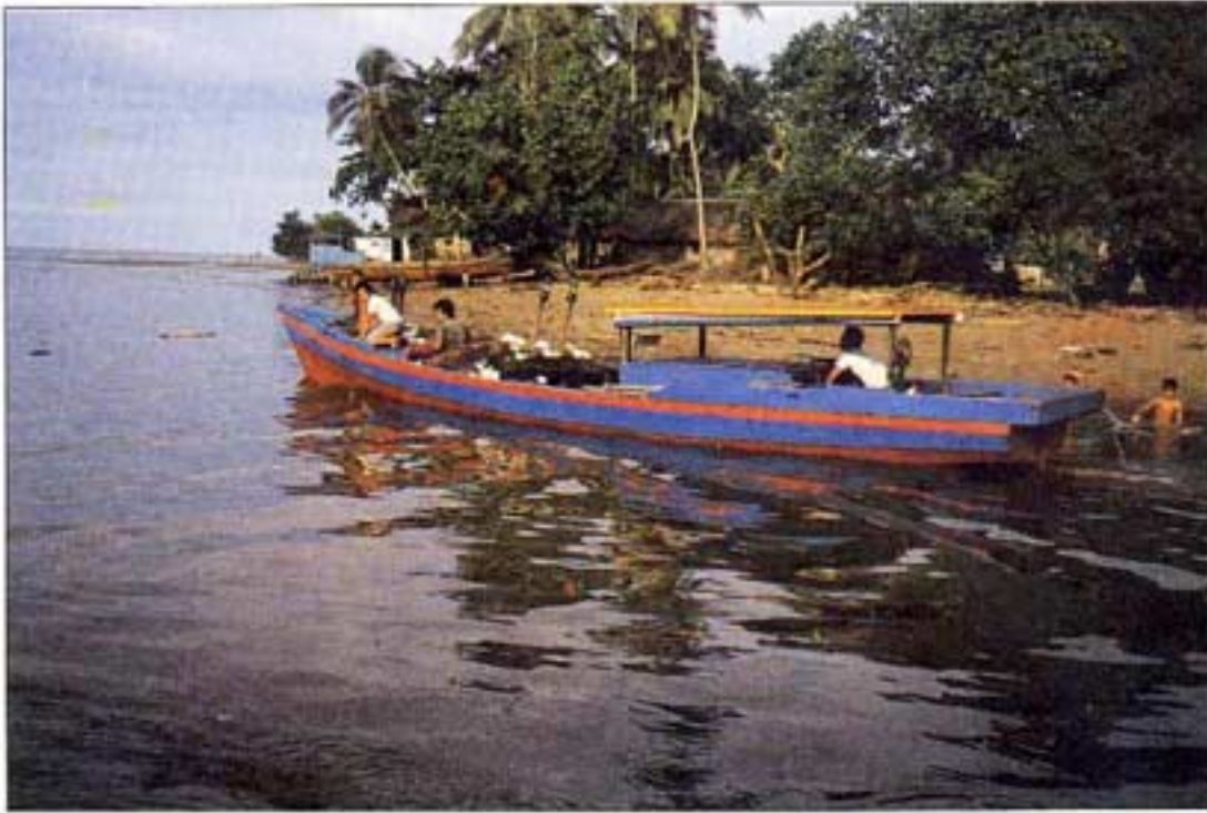
A small inboard motorized half-deck driftnetter (8 m)
