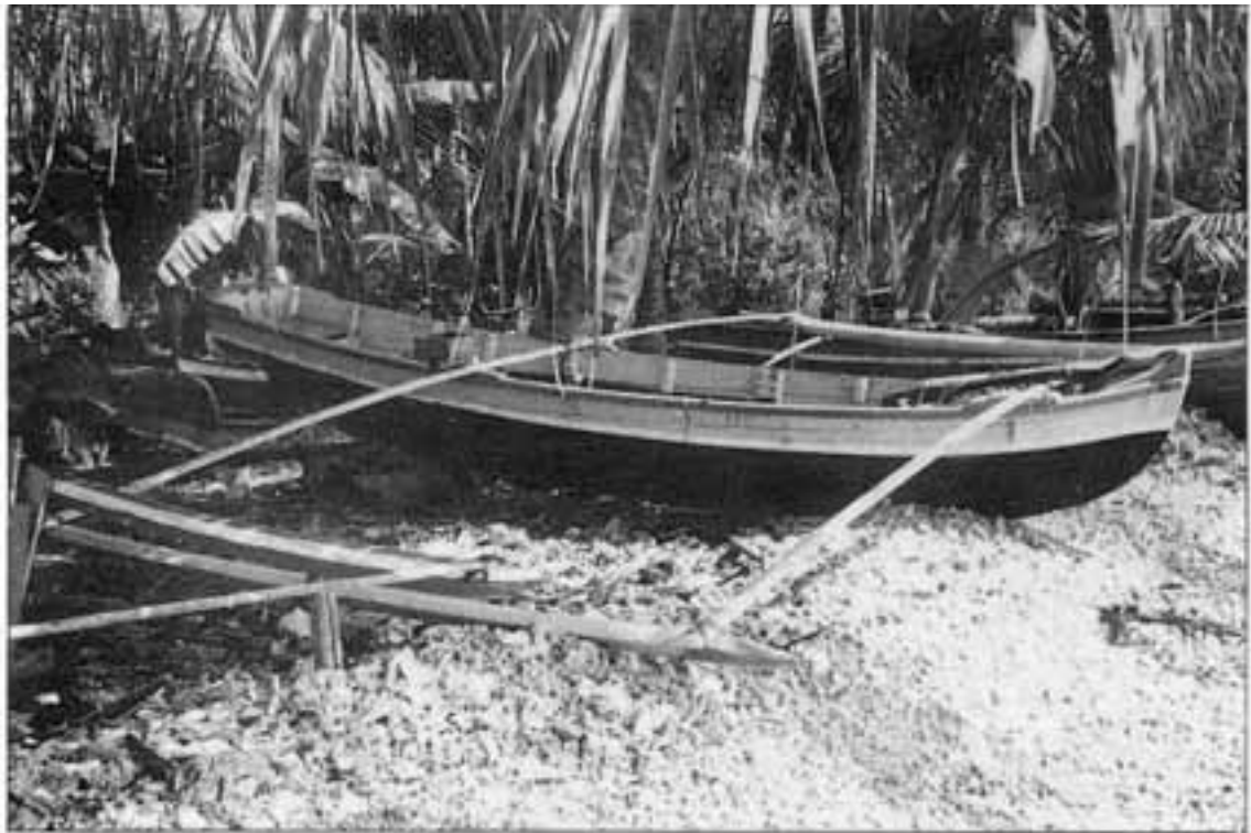
Outboard motorized dugout outrigger canoe (5-7 m)
