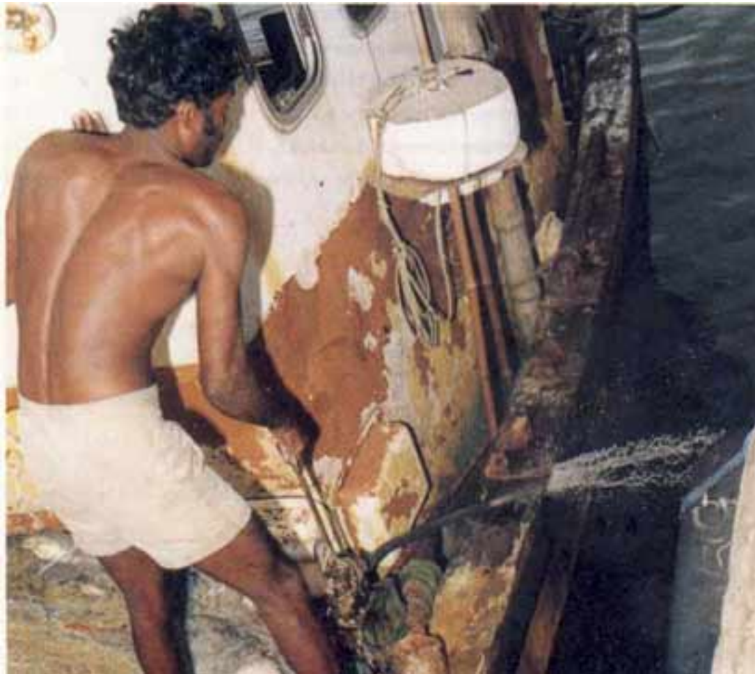
The two commonest causes of pollution in fishery harbours: (1) lack of reception facilities for garbage, resulting in it being dumped into harbour waters (above), and pumping of oily bilge water into harbour waters (below).
