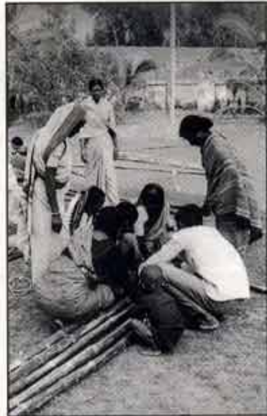
Trainees assembling the bamboo frame for a cage
