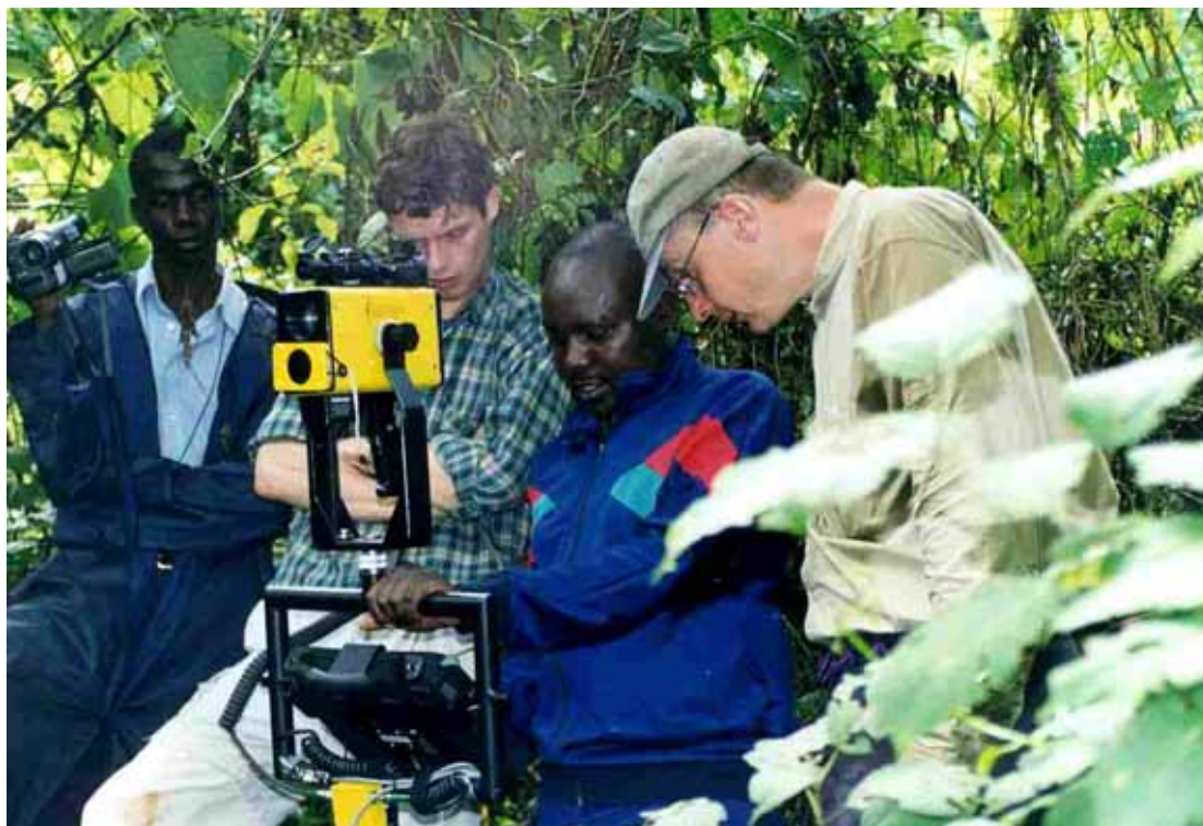
Figure 8: The Field-Map system in use for measurement of biomass in sample plots. The operator is using a field computer mounted on a monopod, on top of which is a laser range finder. The operator is entering data with an electronic pen into the Field-Map database. It will be downloaded later to a PC in the office
