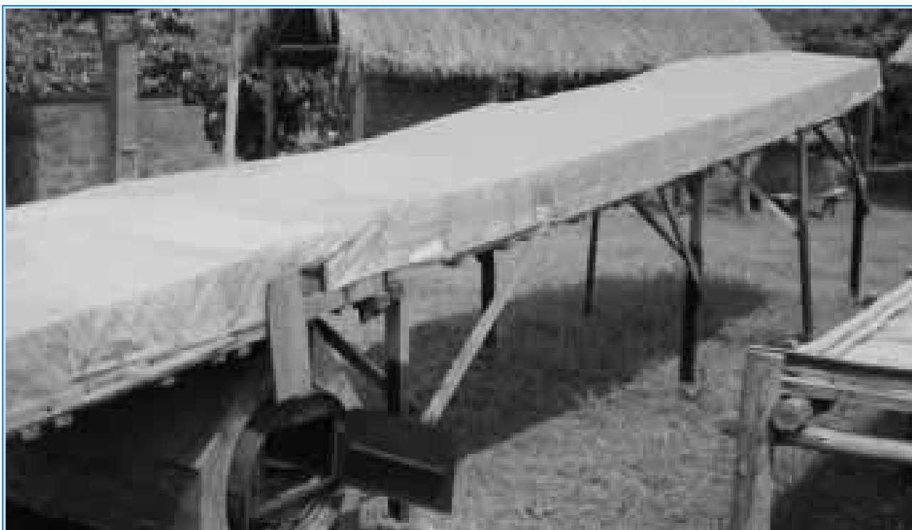
FIGURE 6 Combined solar and fuel-fired dryer. (Photo by the author)
