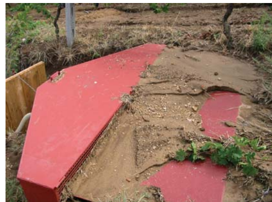
Plate 1 Soil particles obstructing the grating of the trapping system in the conventional treatment.
