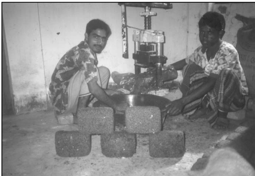
Figure 6.3 A mechanical device being used for making UMMB licks.
