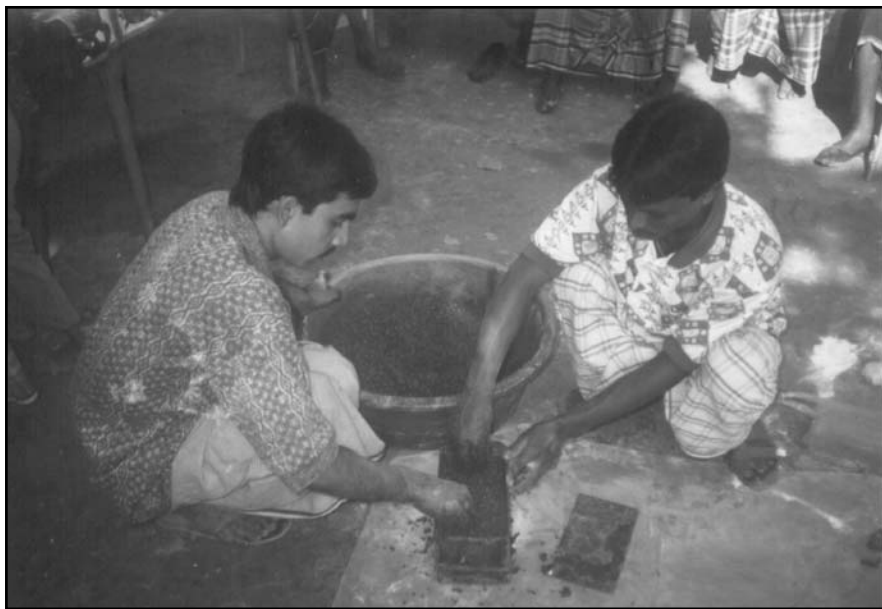
Figure 6.2 Placing the mixture into a mould.
